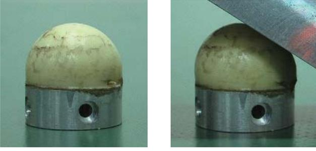
Fig. 3. Soft finger and Contact situation.
