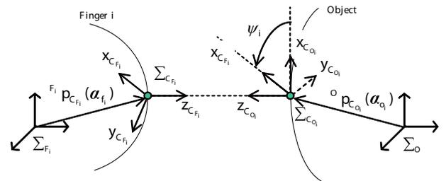
Fig. 5. Contact coordinates before the deformation.
