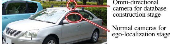
Fig. 9. The vehicle equipped with Omni I and the normal cameras.
