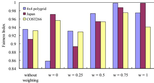
Fig. 6. Effect of weighting in three topologies:  $L_{amp}$  is 1.0, no rerouting
