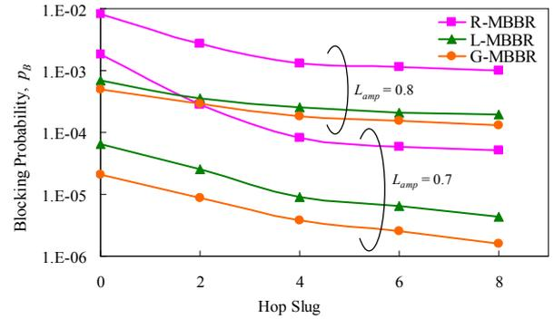
Fig. 11. Effect of hop-slug restriction in 4x4 polygrid network
