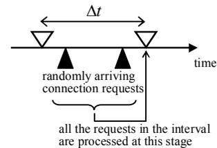
Fig. 1. Periodic path connect/disconnect operations
