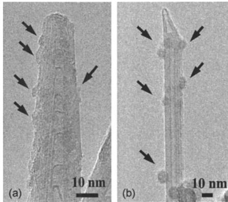
FIG. 3. TEM images of Al-deposited MWNTs (a) before and (b) after field emission. Mean thickness of deposited Al is 2.5 nm. Arrows indicate Al clusters. Different MWNTs are shown in (a) and (b) because we could not find the same MWNT before and after the emission measurement.
