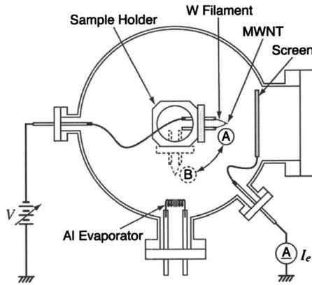
FIG. 1. Schematic of the FEM and metal deposition chamber.
