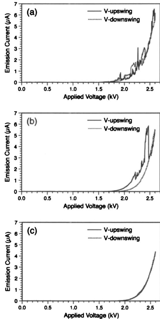
FIG. 2.  $I$ - $V$  curves: (a) Prior to Al deposition, (b) the first run after Al deposition, and (c) the second run after Al deposition.
