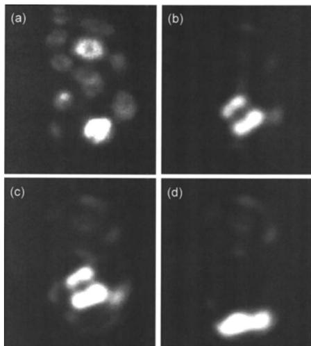
FIG. 4. Time-sequential series of FEM images of a MWNT emitter. (a) Before Al deposition and (b)–(d) after Al deposition. Time elapsed from (b) to (c) is 3.34 s, and that from (c) to (d) is 0.13 s. The voltage applied to the emitter is 1.5 kV.
