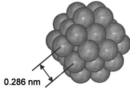
FIG. 5. Cubo-octahedron of an  $\text{Al}_{38}$  cluster.
