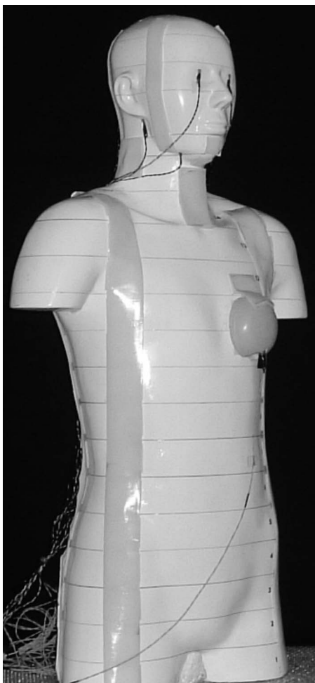
FIG. 2. An anthropomorphic phantom dosimetry system. Seen with the phantom are twisted carbon-fiber cables derived from photodiode dosimeters embedded within the phantom.
