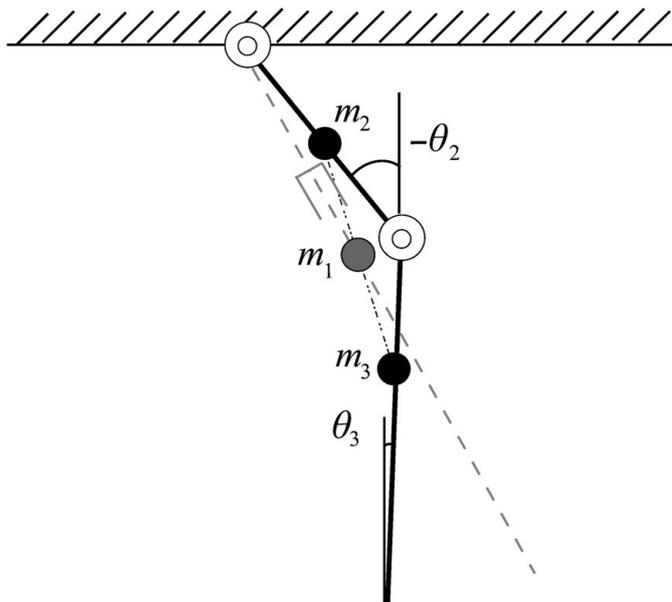
Fig. 5. Double pendulum and its equivalent one-link model with prismatic joint.
