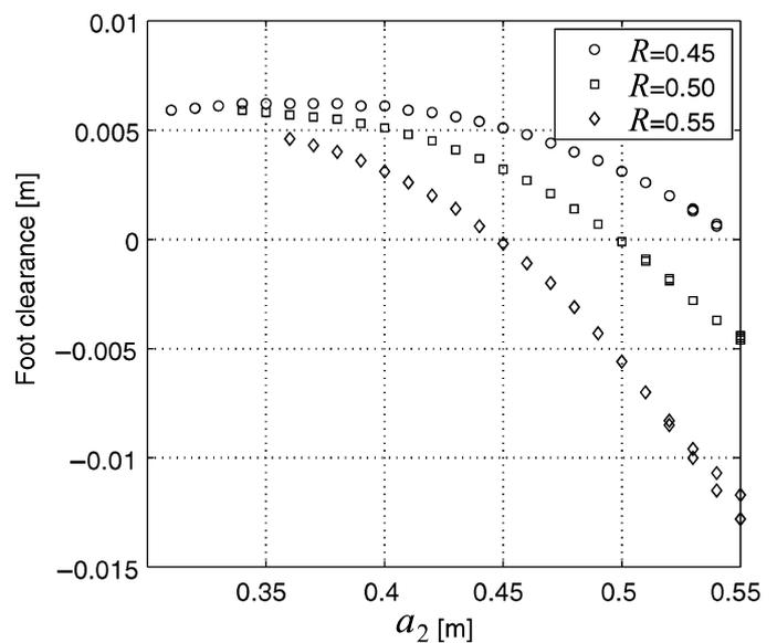
Fig. 12. Foot clearance with respect to  $a_2$ .
