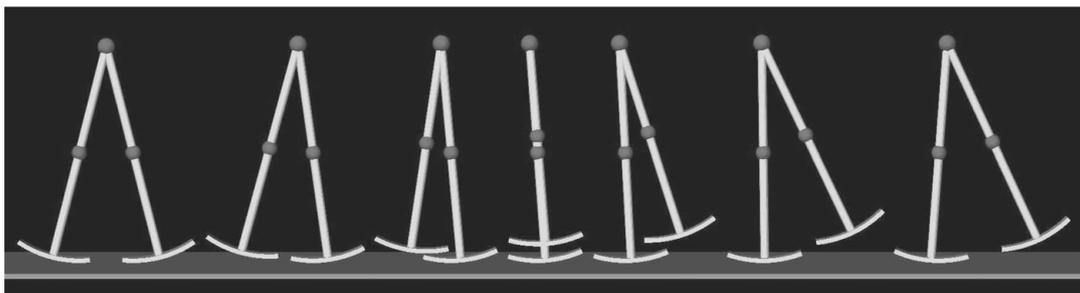
Fig. 4. Parametrically excited dynamic bipedal walking by swing-leg actuation.
