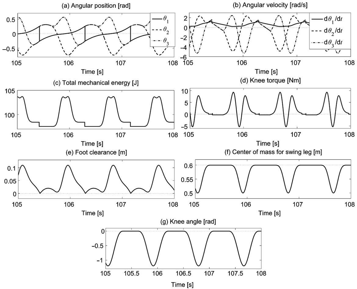
Fig. 10. Simulation results for steady gait pattern.
