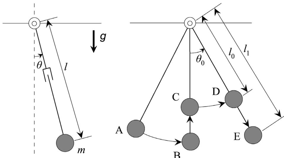
Fig. 2. Optimal trajectory of pendulum in parametric excitation.
