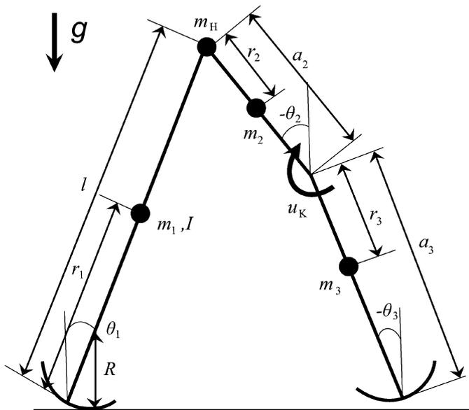
Fig. 1. Model of planar kneed biped robot with semicircular feet.
