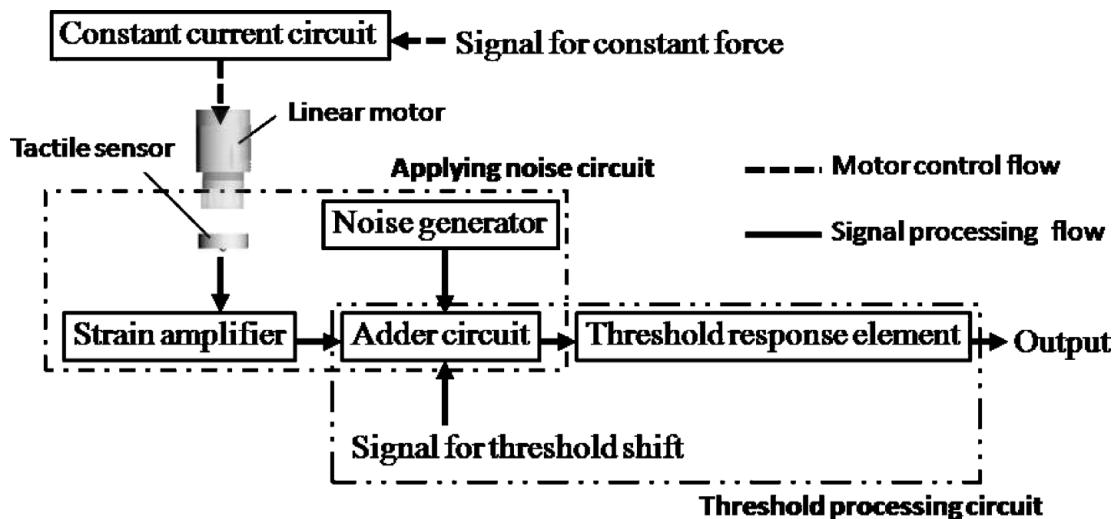
Fig. 8. Schematic block diagram of circuit generating SR.
