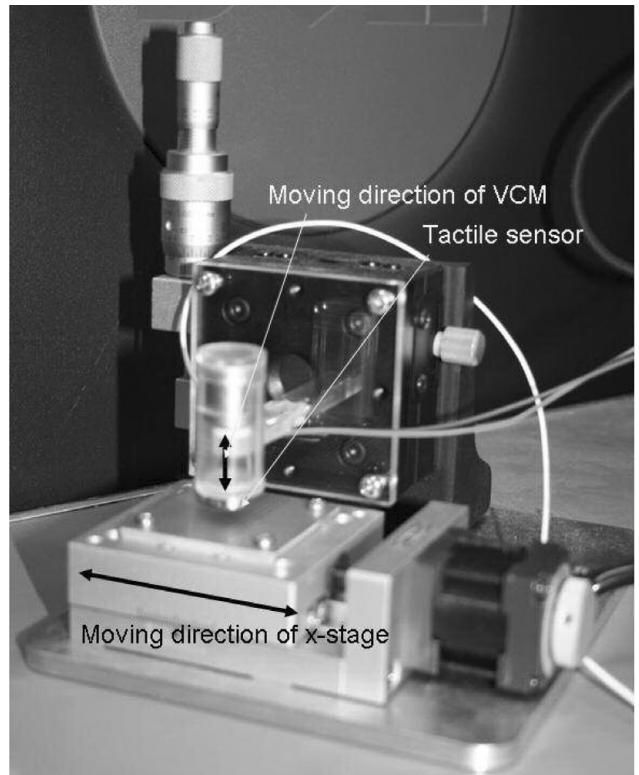
Fig. 1. Scanning testing machine equipped with tactile sensor.
