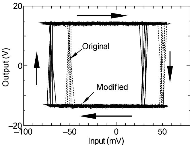
Fig. 9. Limit cycle obtained by Schmitt-trigger circuit.
