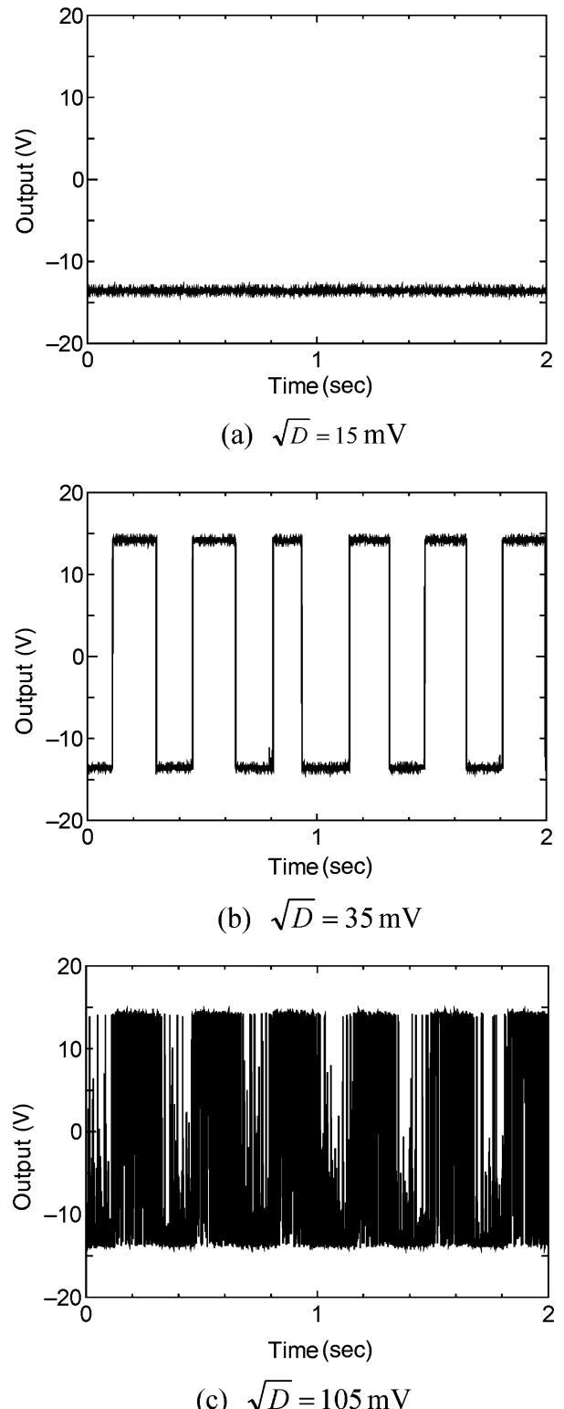
Fig. 11. Output of present circuit (a)  $\sqrt{D} = 15 \text{ mV}$ , (b)  $\sqrt{D} = 35 \text{ mV}$ , (c)  $\sqrt{D} = 105 \text{ mV}$ .
