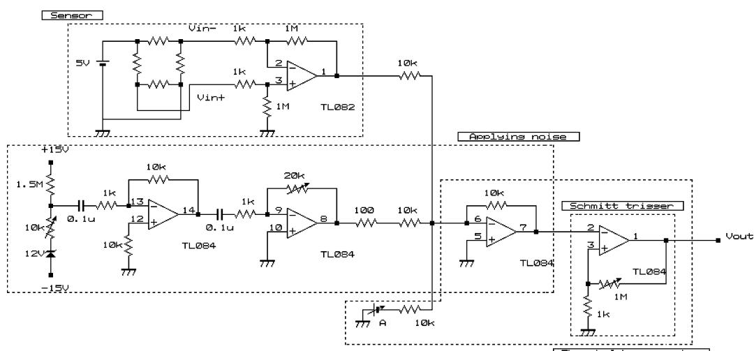
Fig. 12. Circuit generating SR including Schmitt trigger.
