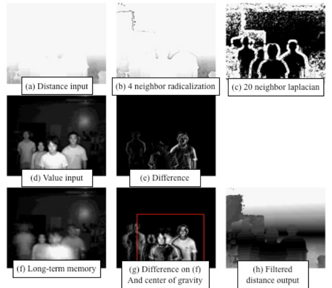
Fig. 2 Digital Image processing for multiple human detection
