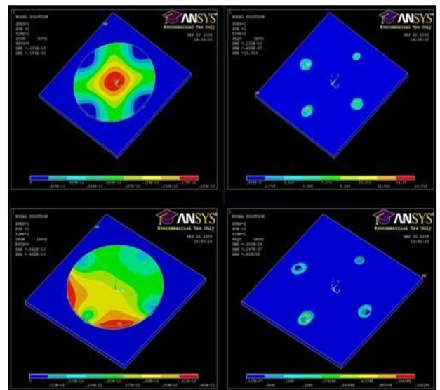
FIG 2. Strain distribution under normal(Z) and shear(Y) load
