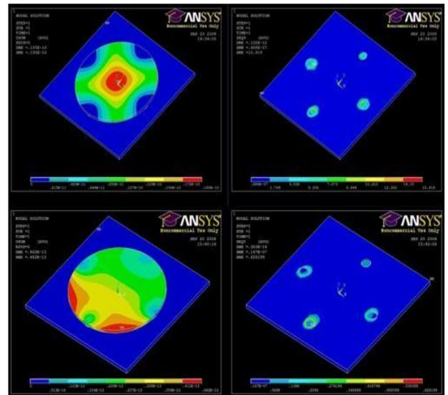
FIG 2. Strain distribution under normal(Z) and shear(Y) load
