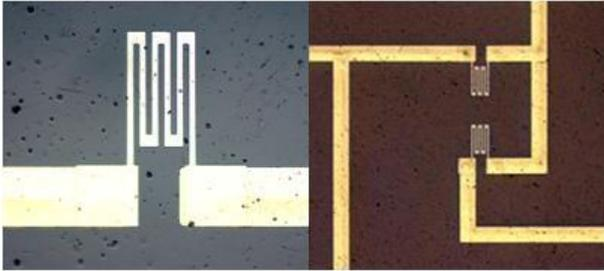
FIG 3. Deposited strain gage and lead line on the polymer substrate
