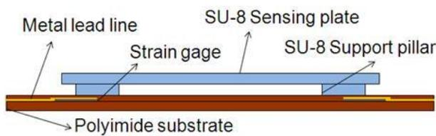
FIG 1. Schematic diagram of the sensing unit.
