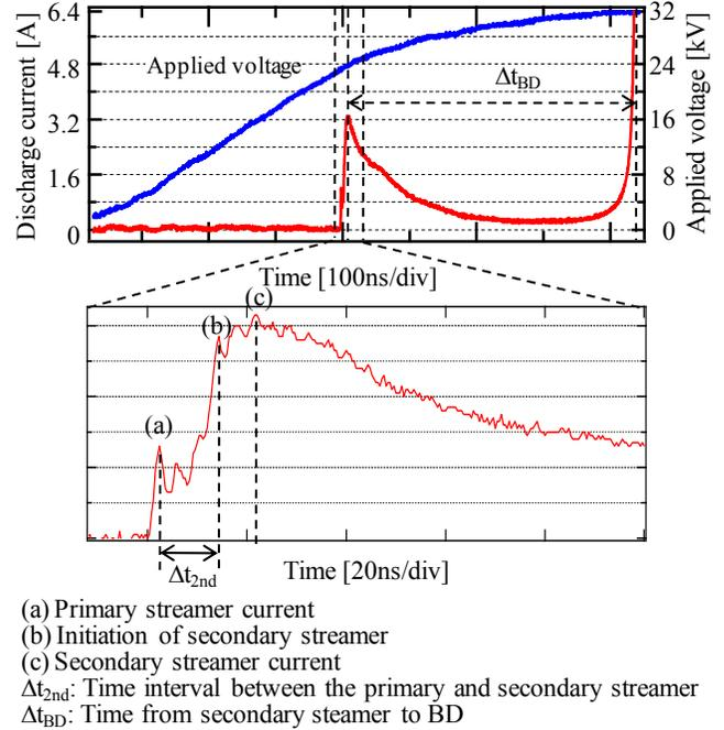
Fig.3 Definition of primary and secondary streamer current and time to BD
