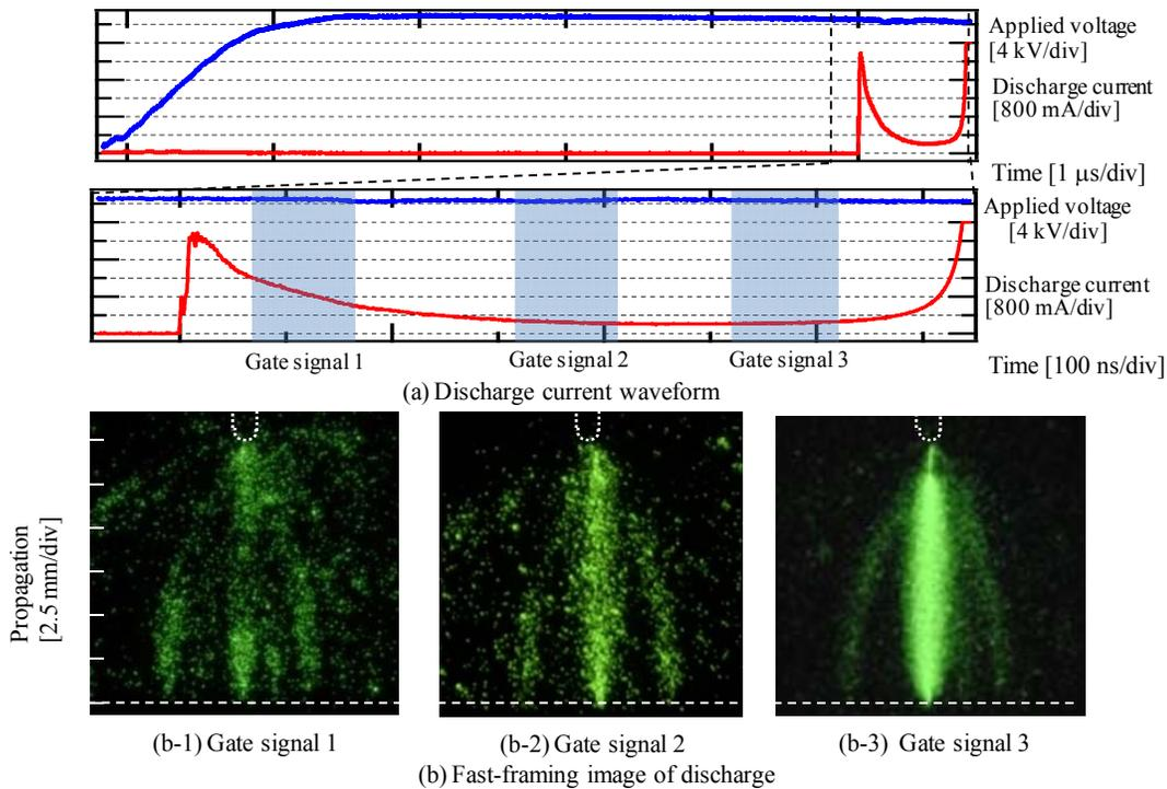
Fig.6 Discharge current waveform and fast-framing images leading to BD ( $V_a = 30$  kV,  $g = 15$  mm)
