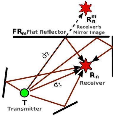
Fig. 1. Many reflected paths with similar path length - problem with finding MPC matching  $FR_m$  reflection. Example of receiver's mirror image concept.
