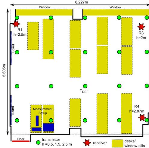
Fig. 5. Experiment Layout. Lecture Room S36, EiTl, PW
