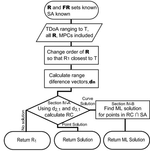
Fig. 3. Flowchart of the proposed algorithm
