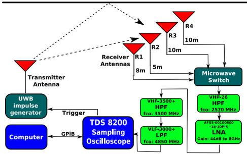
Fig. 4. Measurement Setup, schematic
