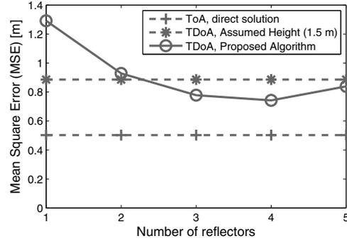
Fig. 6. Average 3D positioning error for different number of known reflectors
