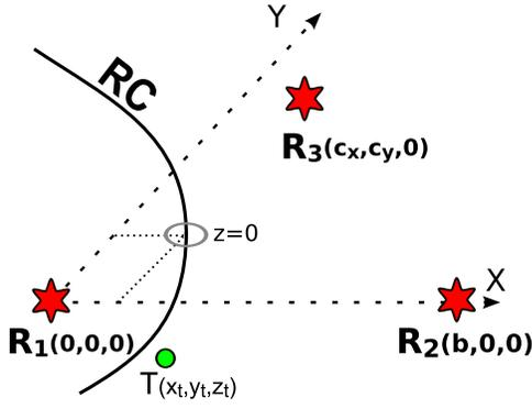
Fig. 2. Result Curve ( $RC$ ) - Second degree curve, solution of eq. (2) for three receivers. Real transmitter position should be near  $RC$ . Presented in prime base.
