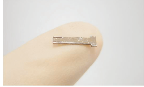
Fig. 11. Fabricated and assembled element for the microarm
