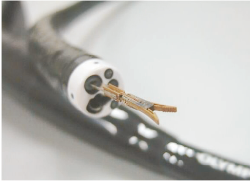
Fig. 12. Developed microarm mounted with an endoscope
