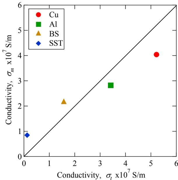
Fig. 11. Comparison of the conductivity,  $\sigma_m$ , obtained by the microwave measurement system and the conductivity,  $\sigma_t$ , measured by high-frequency conductometry.
