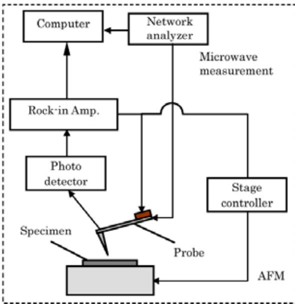
Fig. 3. Configuration of the microwave measurement system.
