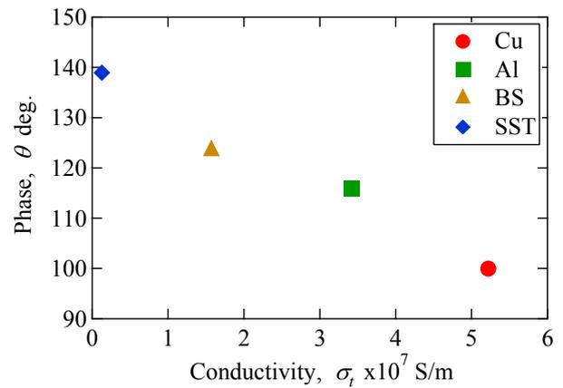
Fig. 10. The phase of the measured reflection coefficient as a function of the electrical conductivity.
