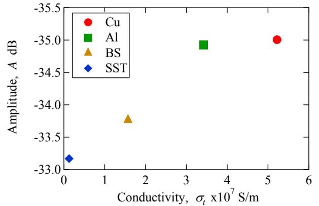
Fig. 9. The amplitude of the measured reflection coefficient as a function of the electrical conductivity.
