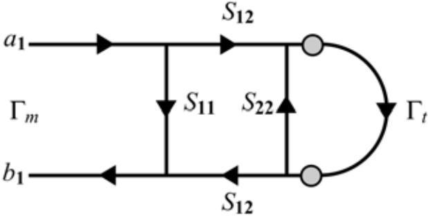
Fig. 2. Signal flow graph of reflection measurement circuit.
