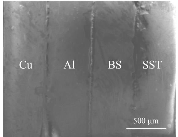
Fig. 5. The SEM photograph of sample which consists of four kinds of metals; the height is 2mm and the width is 0.5 mm, respectively.
