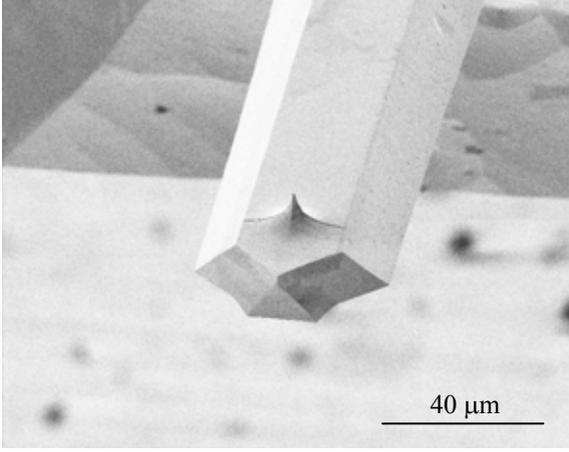
Fig. 1. An M-AFM probe introduced by FIB fabrication.
