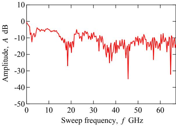
Fig. 6. The amplitude of the reflection coefficient as a function of sweep frequency in free space.
