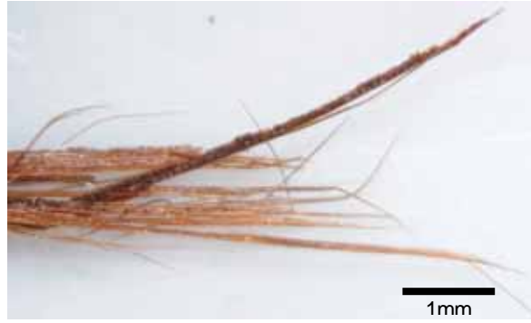
Fig. 6-5 Rupture point of bamboo fiber.
