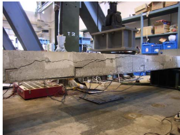
Fig. 4.18 Concrete fracture (L-100)
