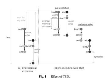
per level in the memory hierarchy. As a result, in the main execution, two loads hit the L1 data cache, resulting in a speedup. Note that in the pre-execution, MLP is improved by overlapping the memory accesses. This further improves the timing of the data fetch in the main execution.
