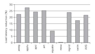
Fig. 10 Load latency reduction rate of TSD-addrpred model relative to TSD model.
