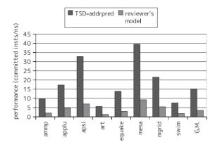
**Fig. A** $\cdot$ **1** Performance (committed instructions per ns) of TSD-addrpred model and base with a register file enlarged by using the transistors for the VHT and DAT.
