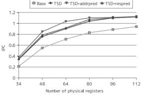
Fig. 6 IPC when varying number of physical registers.
