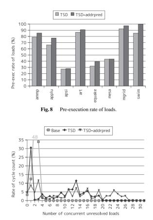
**Fig.9** Distribution of number of unresolved loads whose resolution takes more than or equal to 300 cycles exist simultaneously in art.
