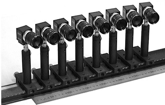
Fig. 1 Multi-view camera system (eight cameras).
