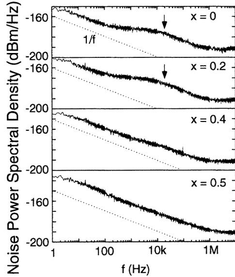
Fig. 7 Low frequency noise spectra of the gate current at room temperature.  $V_{DS}=1.5$  V,  $V_{GS}=0$  V for  $x=0, 0.2, 0.4$  and  $0.5$  for  $x=0.5$ .
