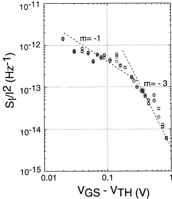
**Fig. 2** Drain-current relative noise spectral density  $S_I/I^2$  at 10 Hz as a function of the effective gate voltage.  $V_{DS}=0.3$  V.
