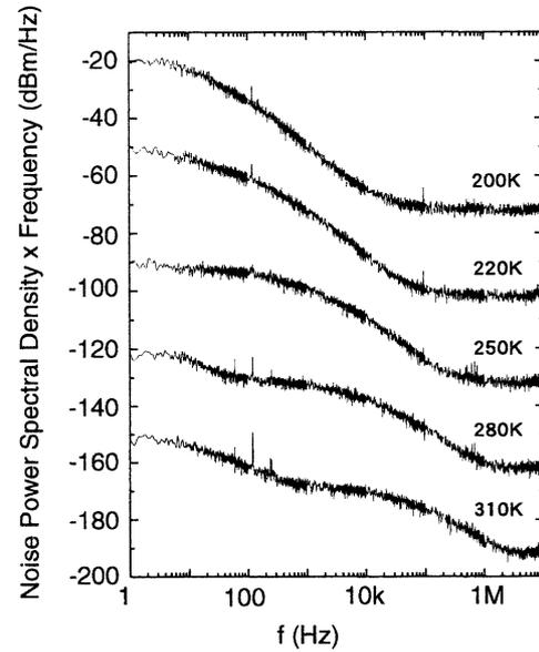
**Fig. 4** Temperature dependence of the drain current noise spectra.
