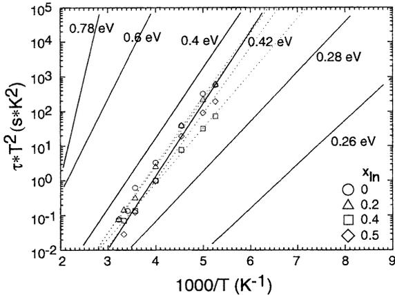
Fig. 6 Arrhenius plots of the time constant of the drain current noise. Solid lines are the deep levels of other reports.
