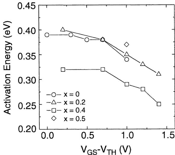
Fig. 9 Activation energy as a function of the effective gate voltage.
