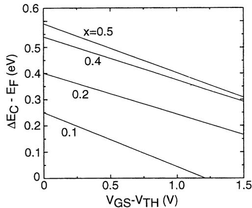
Fig. 10 Calculated barrier height for the real-space transfer as a function of the effective gate voltage.
