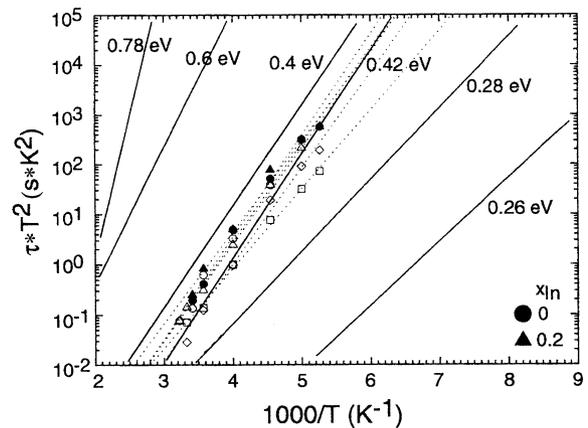
Fig. 8 Arrhenius plots of the time constant of the gate current noise. Solid symbols: gate current noise, open symbols: drain current noise.
