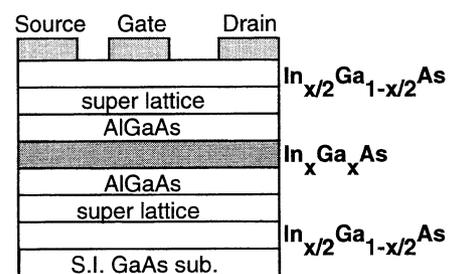
Fig. 1 Schematic cross-section of the AlGaAs/InGaAs pseudomorphic HEMT.
