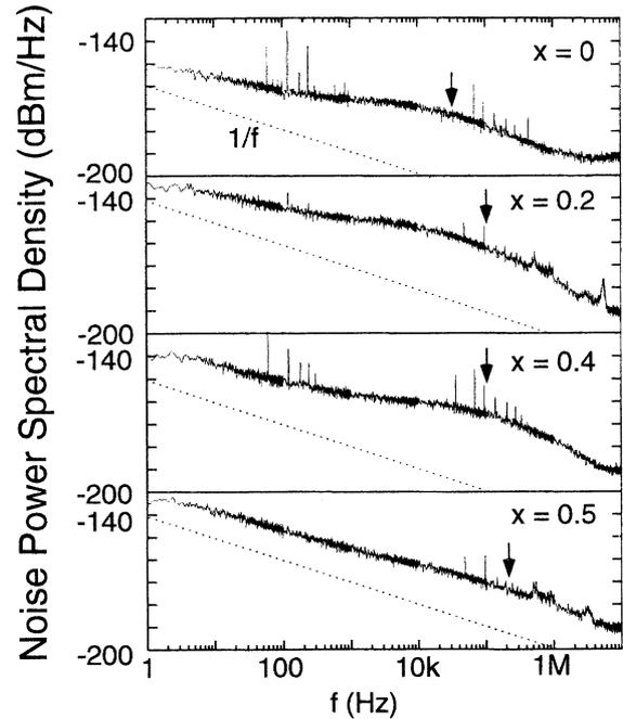
**Fig. 3** Low-frequency noise spectra of the drain current at room temperature.  $V_{DS}=1.5$  V,  $V_{GS}=0$  V for  $x=0, 0.2, 0.4$  and  $0.5$  for  $x=0.5$ .
