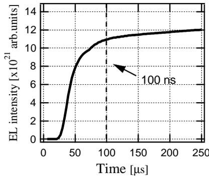
Fig. 7 Time dependence of EL intensity at  $F_a = 140 \text{ MVm}^{-1}$ .
