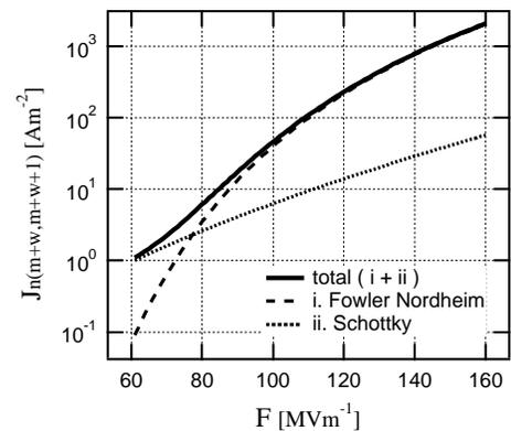
Fig. 11 Field dependence of electron injection.
