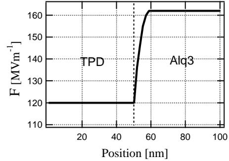
Fig. 5 Distribution of electric field at  $F_a = 140 \text{ MVm}^{-1}$ .
