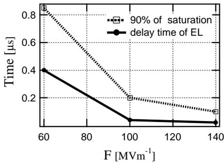
Fig. 8 Field dependence of delay time for luminance.
