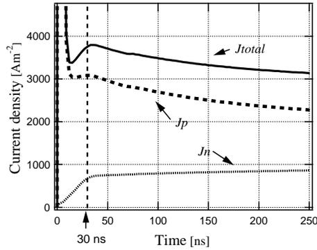
Fig. 6 Time dependence of current densities at  $F = 140 \text{ MVm}^{-1}$ .
