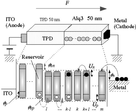
Fig. 1 One-dimensional hopping model.
