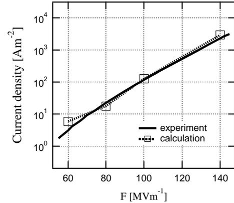
Fig. 9 Field dependence of current density.
