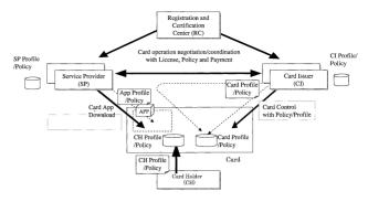
Fig. 2 Dynamic and flexible control using policy and license with profile.
