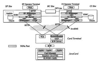
Fig. 4 Prototype system configuration.
