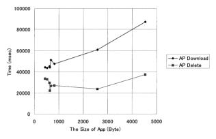
Fig. 8 The time required to download/delete card application.
