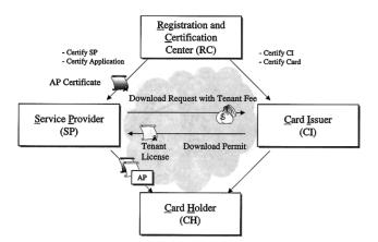
Fig. 1 Role model with an example of typical download sequence.
