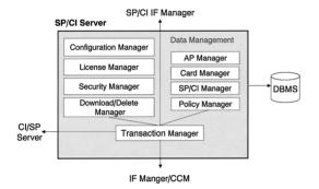
Fig. 5 Software components in SP/CI server.
