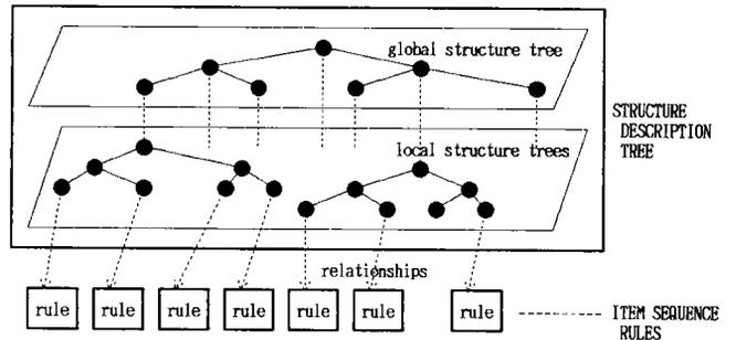
Fig. 10 Relationship between structure description tree and item sequence rules.
