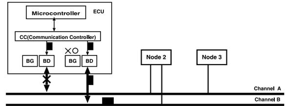
Fig. 2 The node architecture and the dual bus topology configuration.
