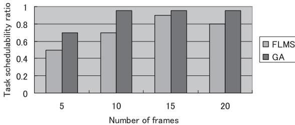
**Fig. 9** Task schedulability ratio comparison between FLMS and GA.
