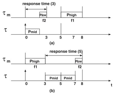
Fig. 3 An example of the critical instant theorem.
