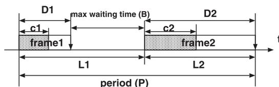
Fig. 1 An I/O blocking task.
