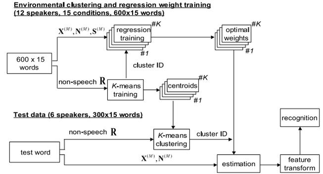
**Fig. 7** Diagram of environmental clustering and regression-based speech recognition.  $\mathbf{X}^{(M)}$ ,  $\mathbf{N}^{(M)}$ , and  $\mathbf{S}^{(M)}$  denote the log MFBC outputs obtained from observed noisy speech, estimated noise, and reference clean speech, respectively.  $\mathbf{R}$  denotes the vector representation of driving environment using Eq. (6).
