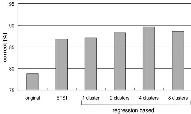
**Fig. 8** Recognition performance for different cluster using adaptive regression methods (averaged over 15 driving conditions).
