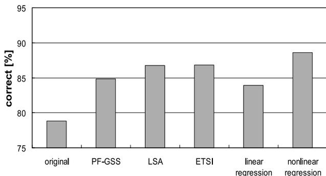
Fig. 5 Recognition performance of different speech enhancement methods (averaged over 15 driving conditions).
