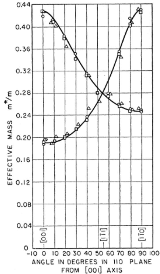
FIG. 6. Effective mass of electrons in silicon at 4°K for magnetic field directions in a (110) plane; the theoretical curves are calculated from Eq. (38), with  $m_2=0.98m$ ;  $m_1=0.19m$ .
