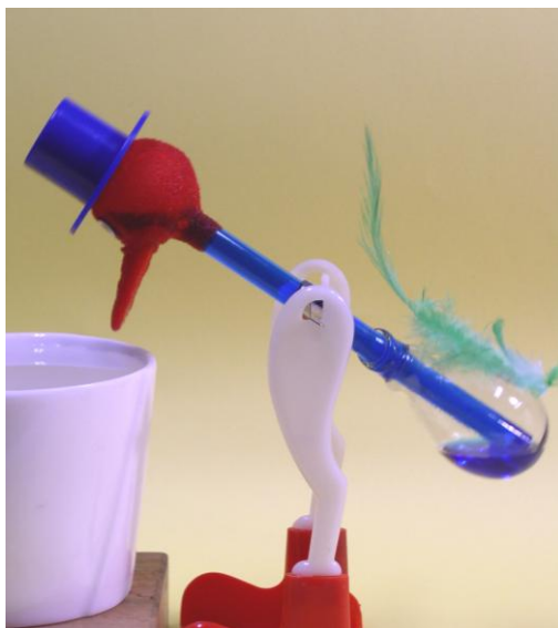
11-5 (a) Drinking Bird as a Heat Engine
