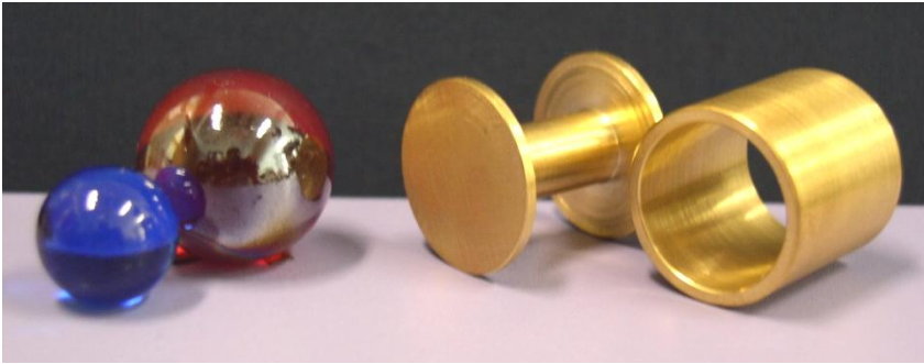
8-2(d) 大小の球、及び 同じ直径、同じ重さの「糸巻き」と「パイプ」の比較 Left; The radius of spheres are different. Right; The radius of a Pipe and a Bobbin are the same.
