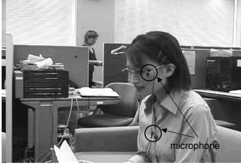
Figure 6: Recording scene - A lavalier microphone is placed on the subjects shirt around the chest area and the other is on the spectacles frame.
