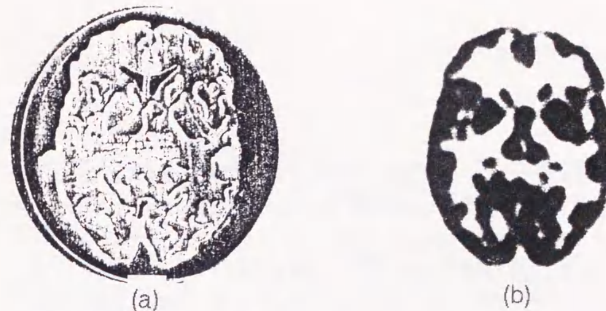
Fig. 3-9. Cross sectional view of the Hoffman brain phantom (a) and an image of the phantom obtained by using the PET(b).
