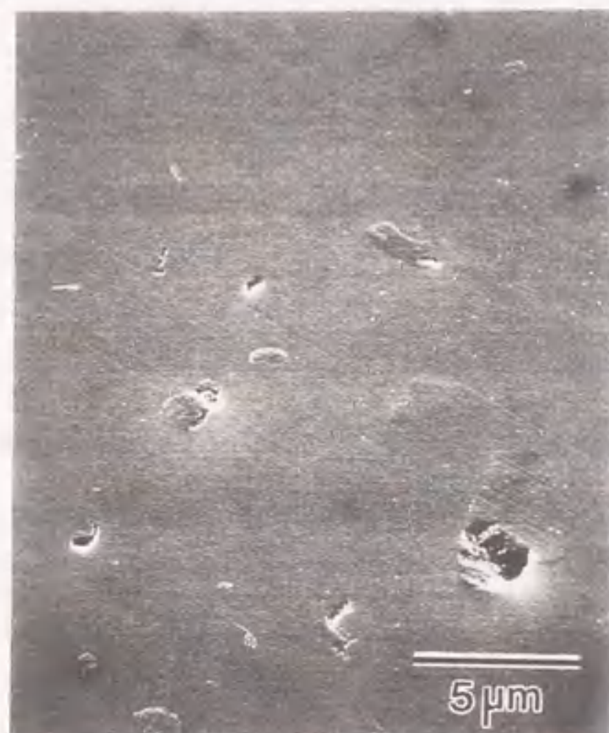
Fig.4-3 Scanning electron micrograph of the worn surface of SiC plate tested at sliding speed of 0.11m/s in water at 300°C.
