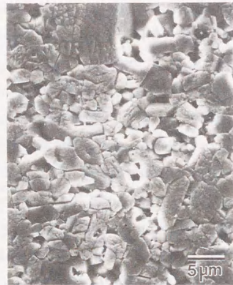
Fig.2-10 Scanning electron micrographs of the surface of ALO-1 soaked in water at 300 °C for 200h.
