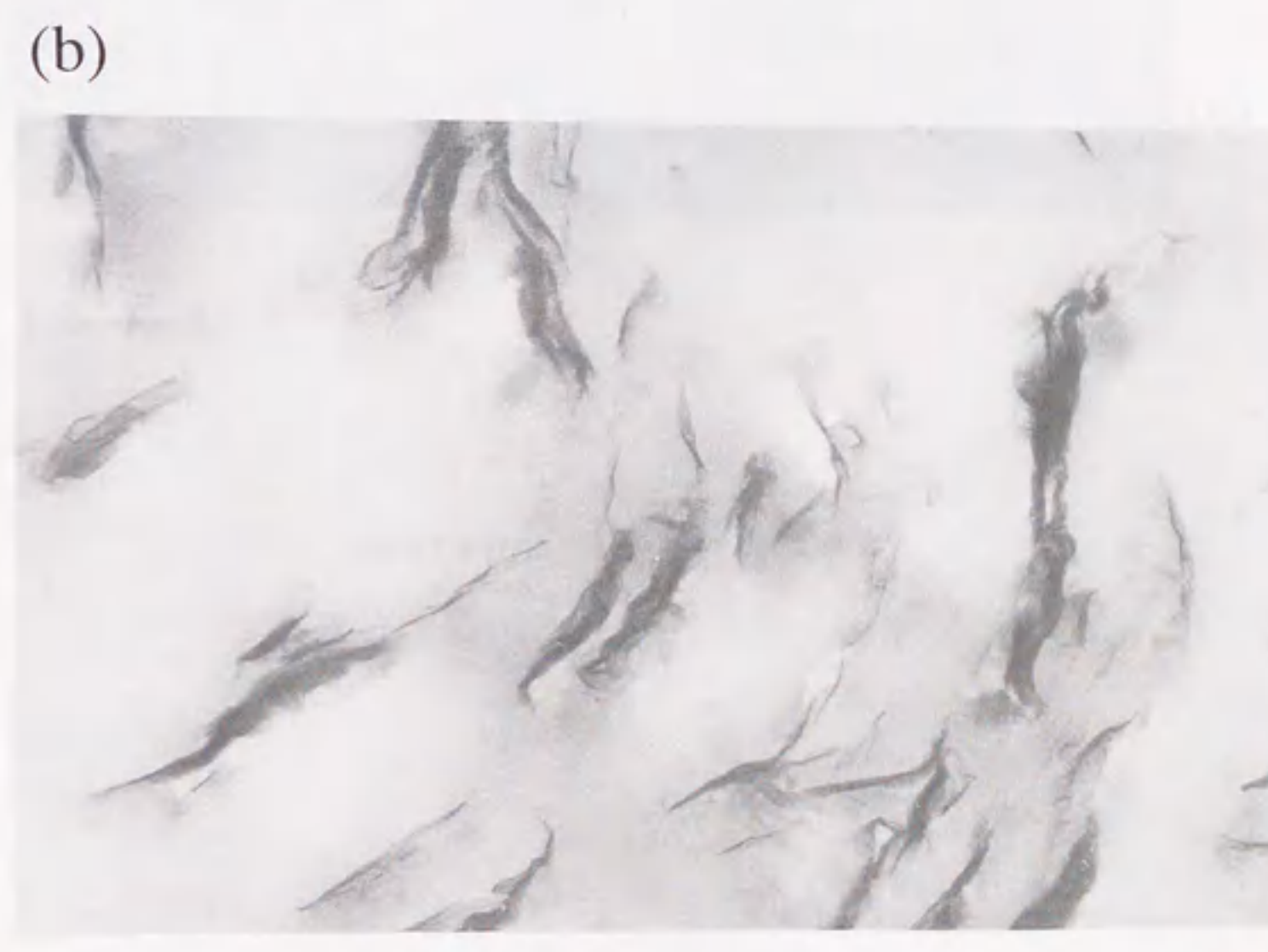
Fig.10-15 TEM photographs of (a): Na-montmorillonite/polypropylene (b) DSDM-montmorillonite/polypropylene (c) PTDA-montmorillonite/polypropylene
