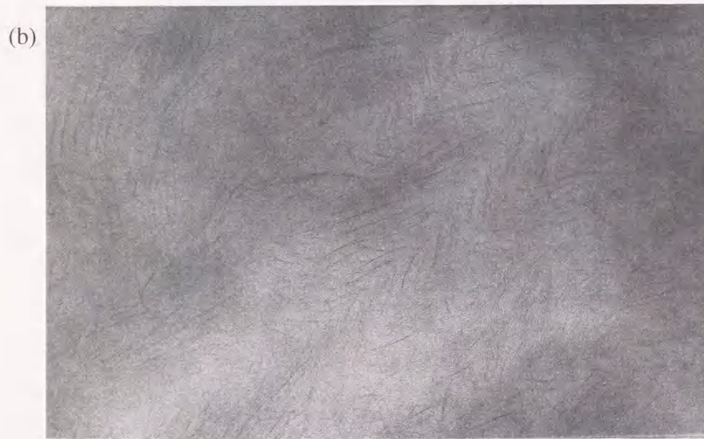
Fig. 3-4 Transmission electron micrographs of section of NCH : (a) 5.3 wt% montmorillonite, (b) 11.3 wt%, (c) 18.2 wt%, and (d) 31.4 wt%.
