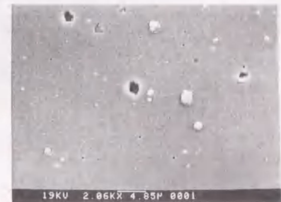
TiN plated SKD11 block (Ra=220nm)
