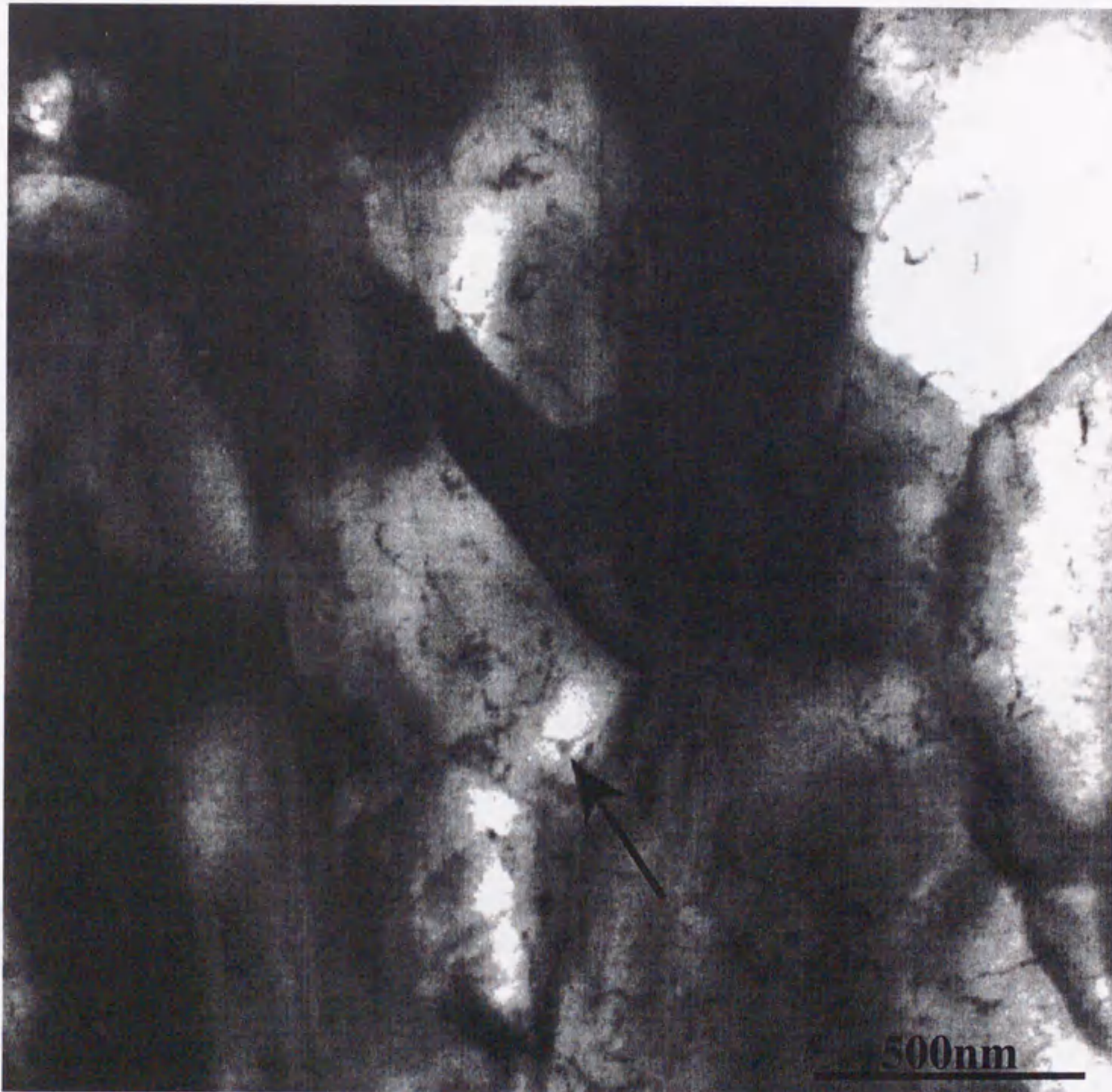
Fig.3-20 A middle layer composed of fine \delta_1 grains in the GA coating.
