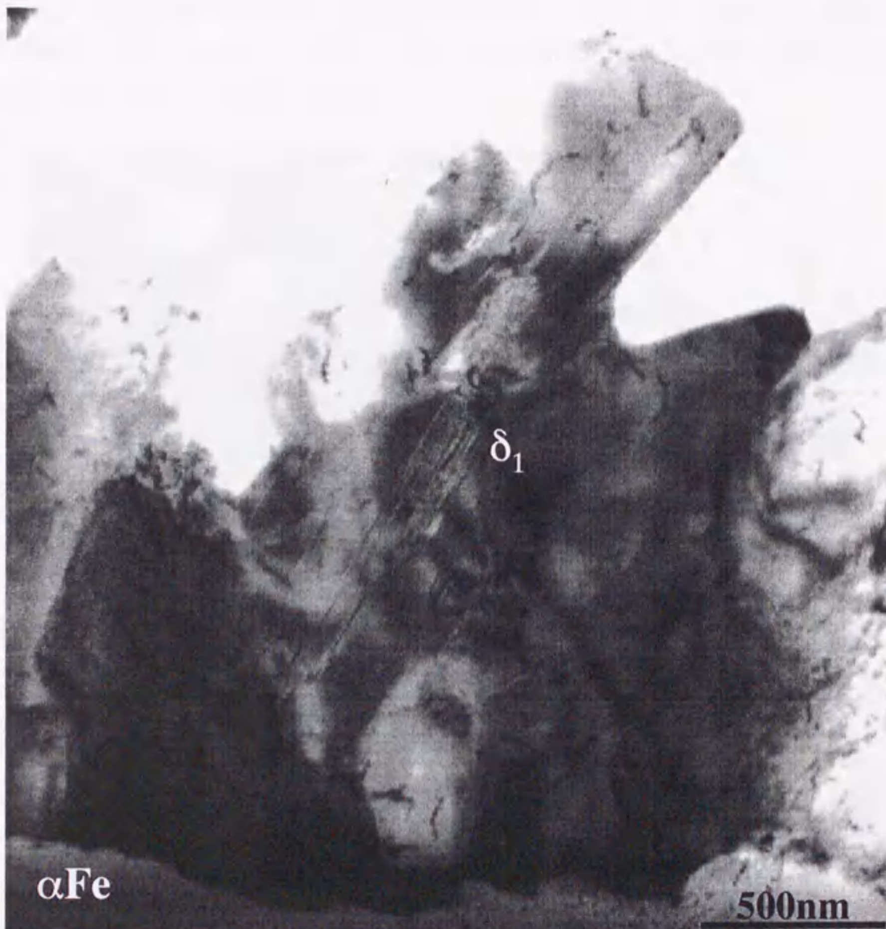
Fig. 4-6 \delta_1 phase formed at an interface between the substrate and the GI coating.
