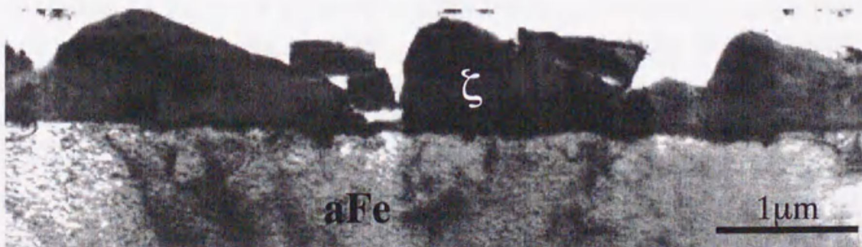
Fig.4-11 Typical epitaxial growth of \zeta phase from the substrate.
