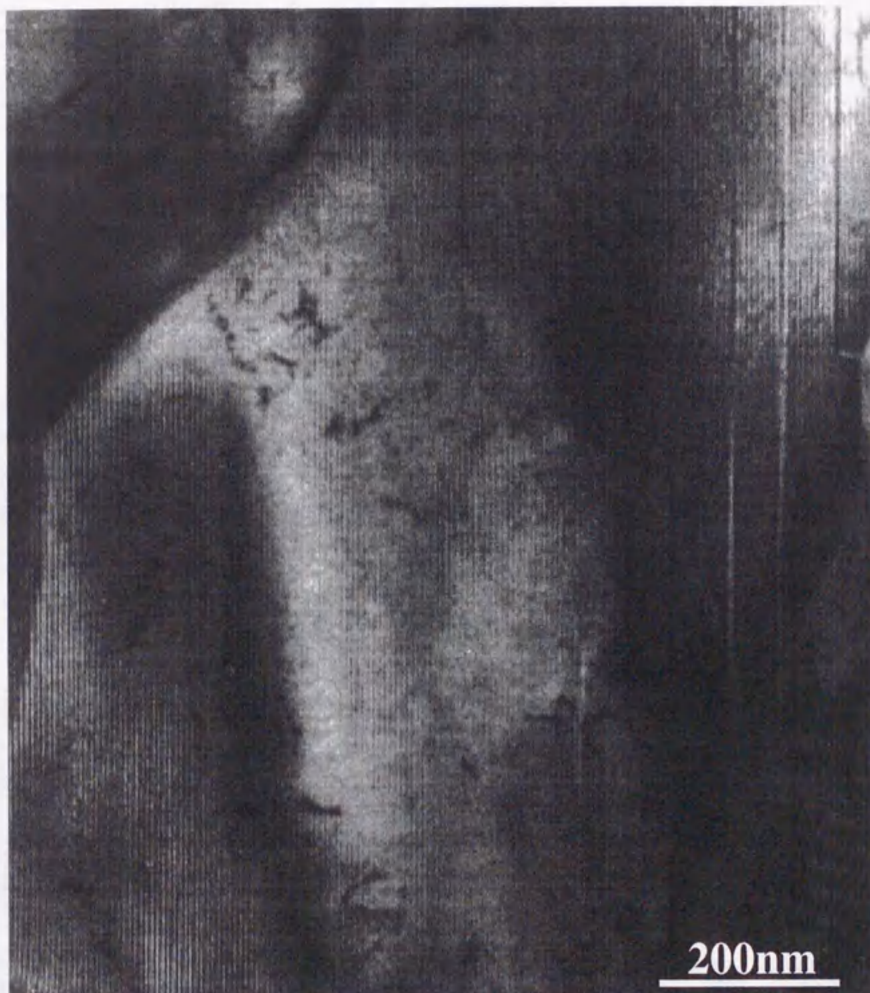
Fig.3-7 Typical \delta_1 phase. Lattice fringes of c plane are observed at a low magnification (spacing c plane= 5.735nm).
