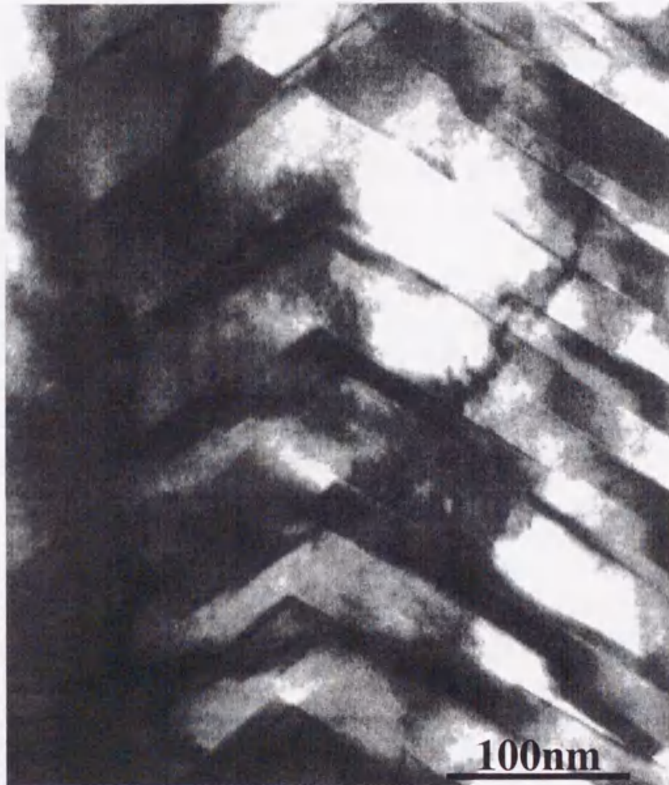
Fig.3-6 Typical \Gamma_1 phase in a GA coating. \Gamma_1 phase contains a high density of liner defects.
