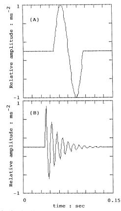
Fig. 1. Acceleration time histories achieved on handle of vibrator. (A) one complete cycle of a 100 Hz sine wave; (B) exponential decay waveform.
