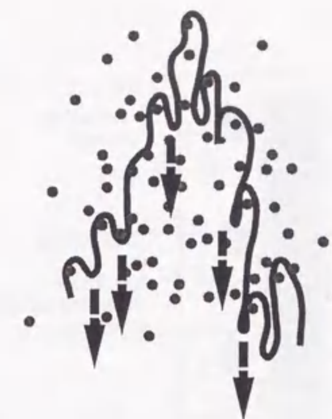
Figure 6.1 A schematic picture of a new theoretical model of gel electrophoresis.
