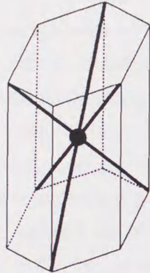
FIGURE 5. The trigonal antiprism ( p^3d^3 hybrids), basic unit for the face-centred cubic structure.
