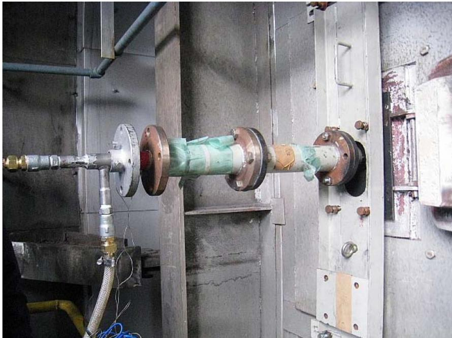
Figure 5-5: Photo of the ash deposition test probe inserted in the boiler.
