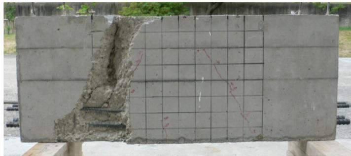
**Fig. 5.7** Failure of BS4bw100
