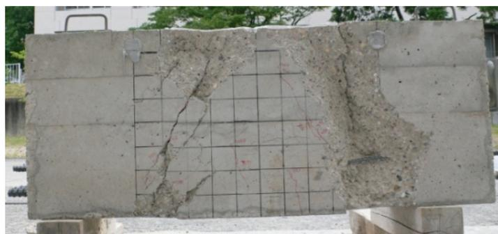
**Fig. 5.9** Failure of BS4bw200
