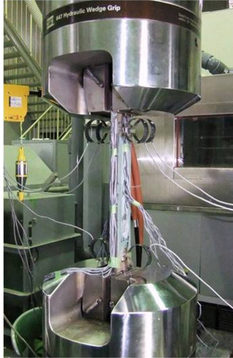
Fig. 6.6 Test setup of CFRP-bonded steel plate
