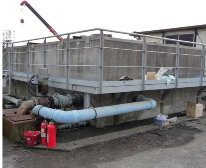
Fig. 2.4 Seawater pool used for underwater welding
