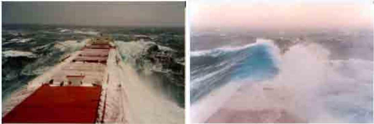
Figure 1.6 Green water on a ship under extreme wave (Source: Buchner, 2007)
