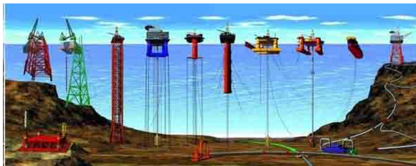
Figure 1.2 Various types of offshore platform (Source: http://en.wikipedia/wiki/Oil-plaform )
