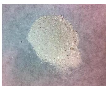
Figure 6.1 Activated oyster shell
