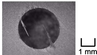
Fig. 6.10 Machined hole viewed from the drill-exit surface
