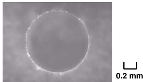
(b) Machined through-hole viewed from the exit surface of the work-piece
