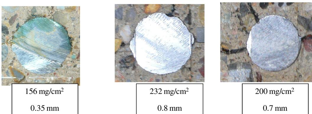
**Figure B.23.** Actual rebar corroded sectional pattern of 150\*150-D25
