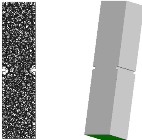
**Figure A.2.** RBSM modeling of "direct" tension specimen
