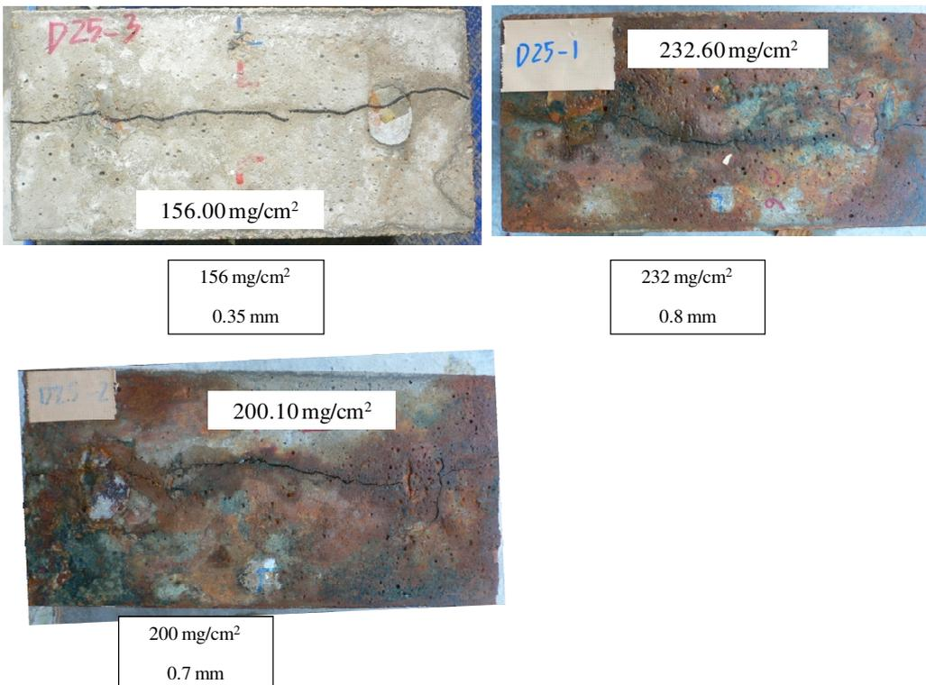
Figure B.21. Surface crack patterns of 150\*150-D25
