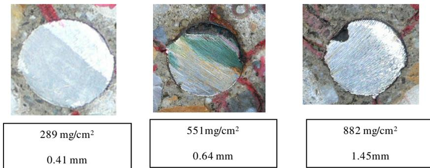
**Figure B.27.** Actual rebar corroded sectional pattern of 300\*150-C30
