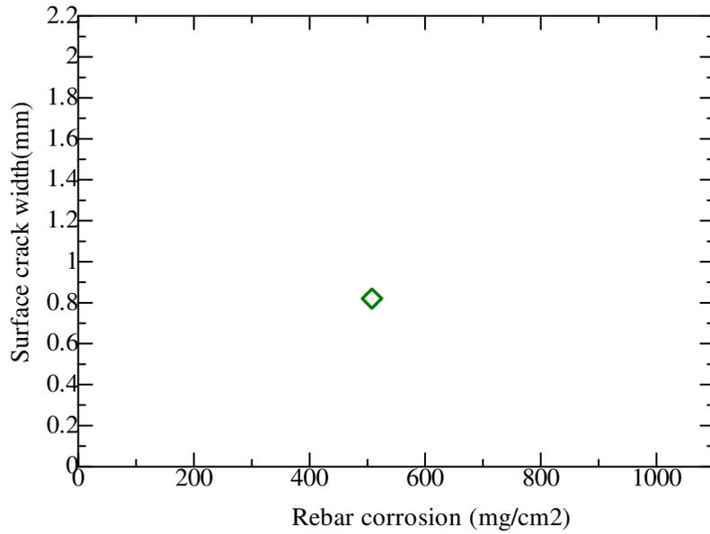
**Figure B.28.** Surface crack width propagation of 250\*250-C30
