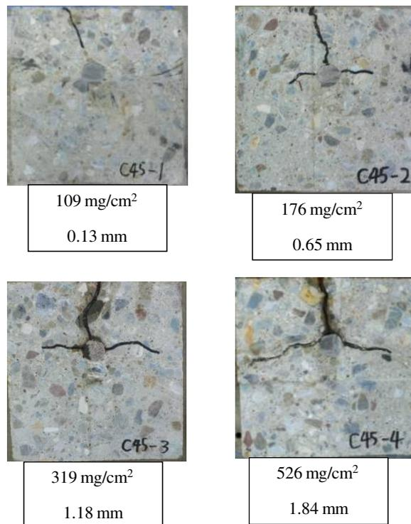
**Figure B.14.** Internal crack patterns of 150\*150-C45
