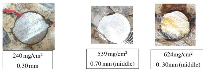
**Figure B.39.** Actual rebar corroded sectional pattern of 600\*400-C30
