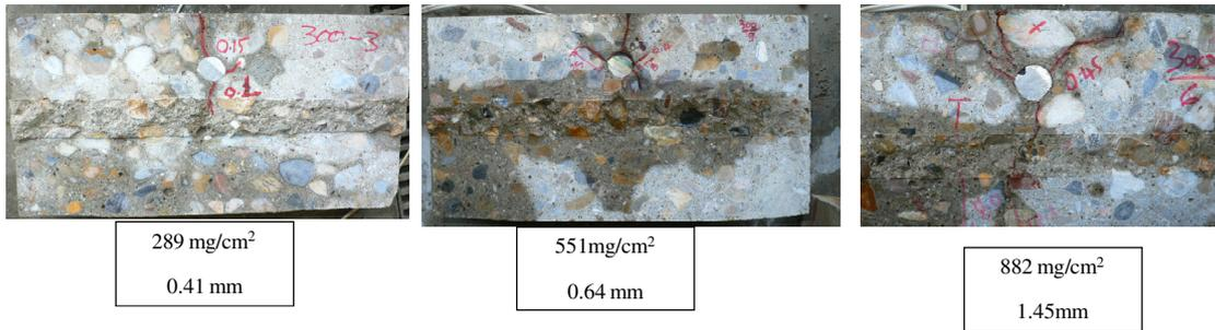
**Figure B.26.** Internal crack patterns of 300\*150-C30
