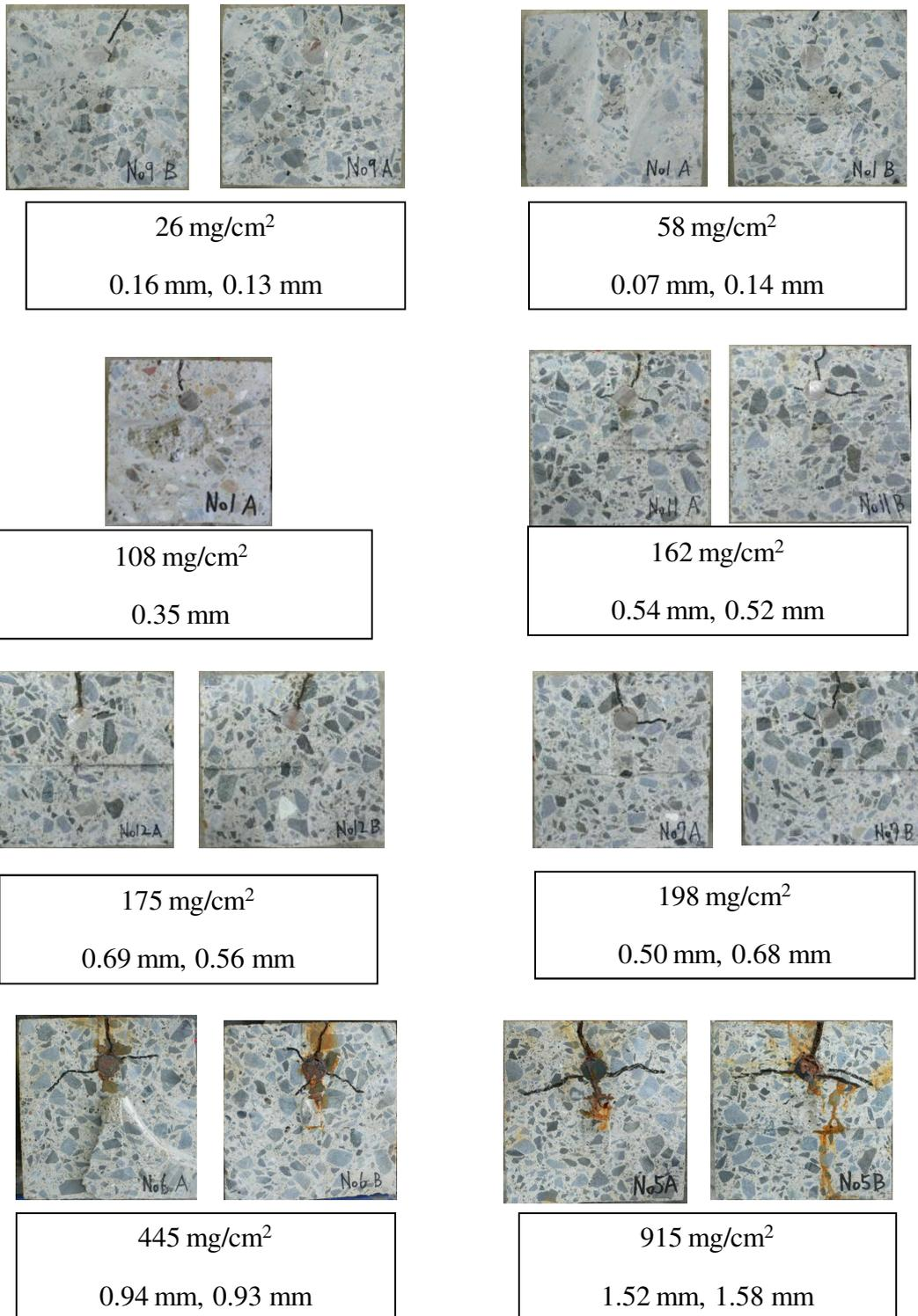
**Figure B.4.** Internal crack patterns of 150\*150-C30
