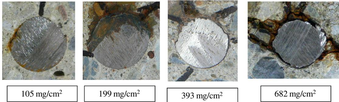
**Figure B.7.** Actual rebar corroded sectional pattern of 150\*150-C7.5
