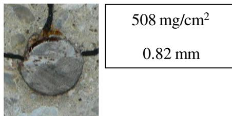
**Figure B.31.** Actual rebar corroded sectional pattern of 250\*250-C30
