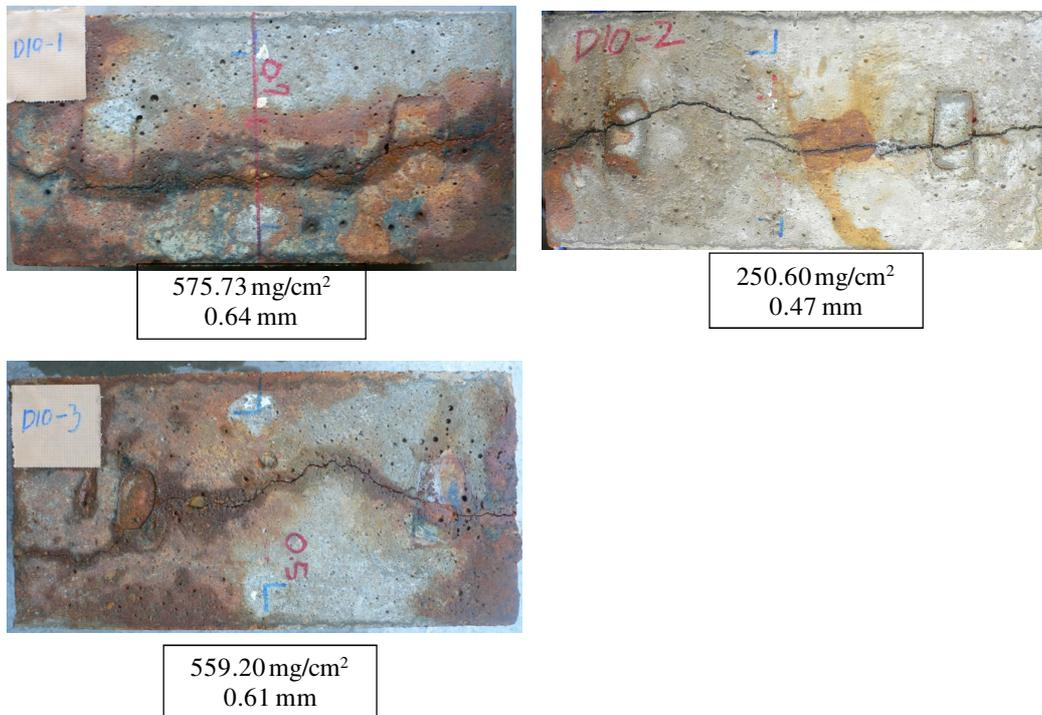
Figure B.17. Surface crack patterns of 150\*150-D10
