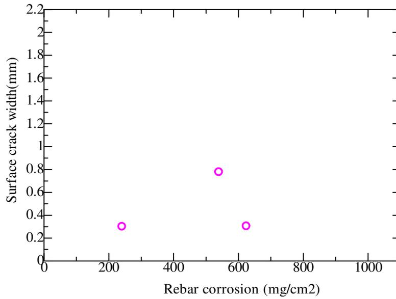
Figure B.36. Surface crack width propagation of 600\*400-C30
