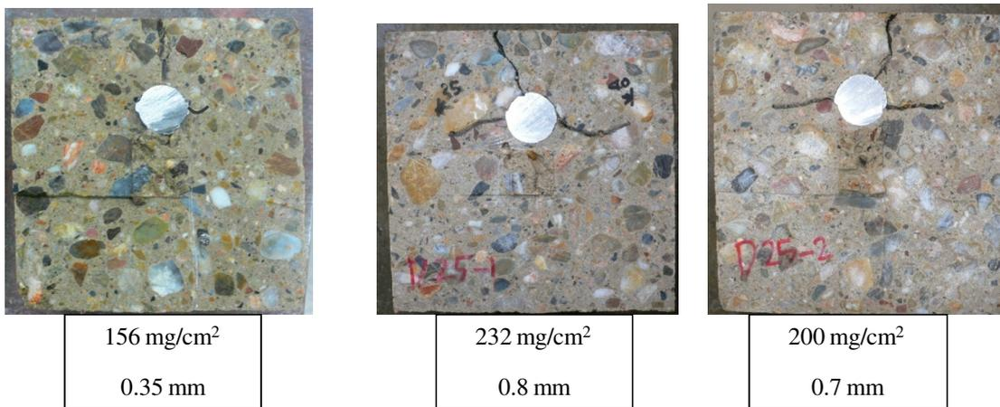
**Figure B.22.** Internal crack patterns of 150\*150-D25
