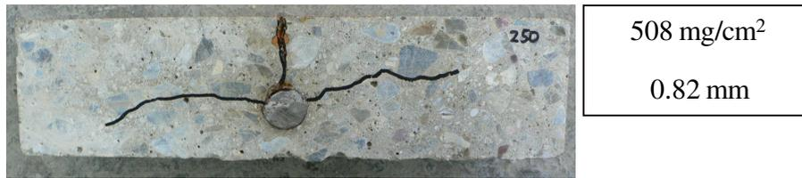
**Figure B.30.** Internal crack pattern of 250\*250-C30
