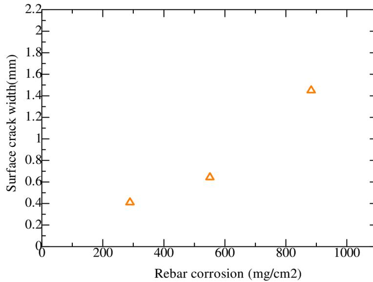
Figure B.24. Surface crack width propagation of 300\*150-C25
