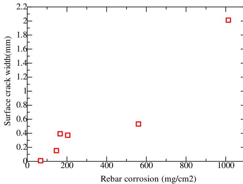
**Figure B.32.** Surface crack width propagation of 400\*400-C30
