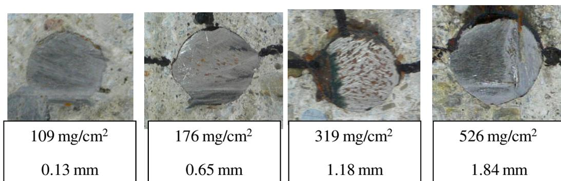
**Figure B.15.** Actual rebar corroded sectional pattern of 150\*150-C45
