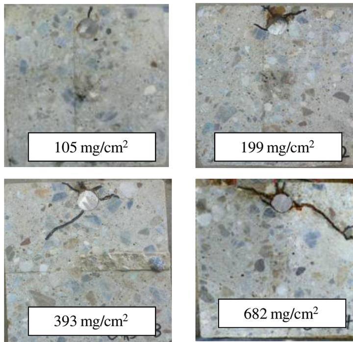
**Figure B.6.** Internal crack pattern of 150\*150-C7.5
