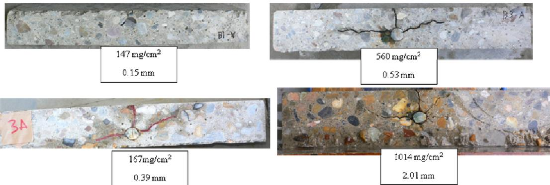
**Figure B.34.** Internal crack pattern of 400\*400-C30
