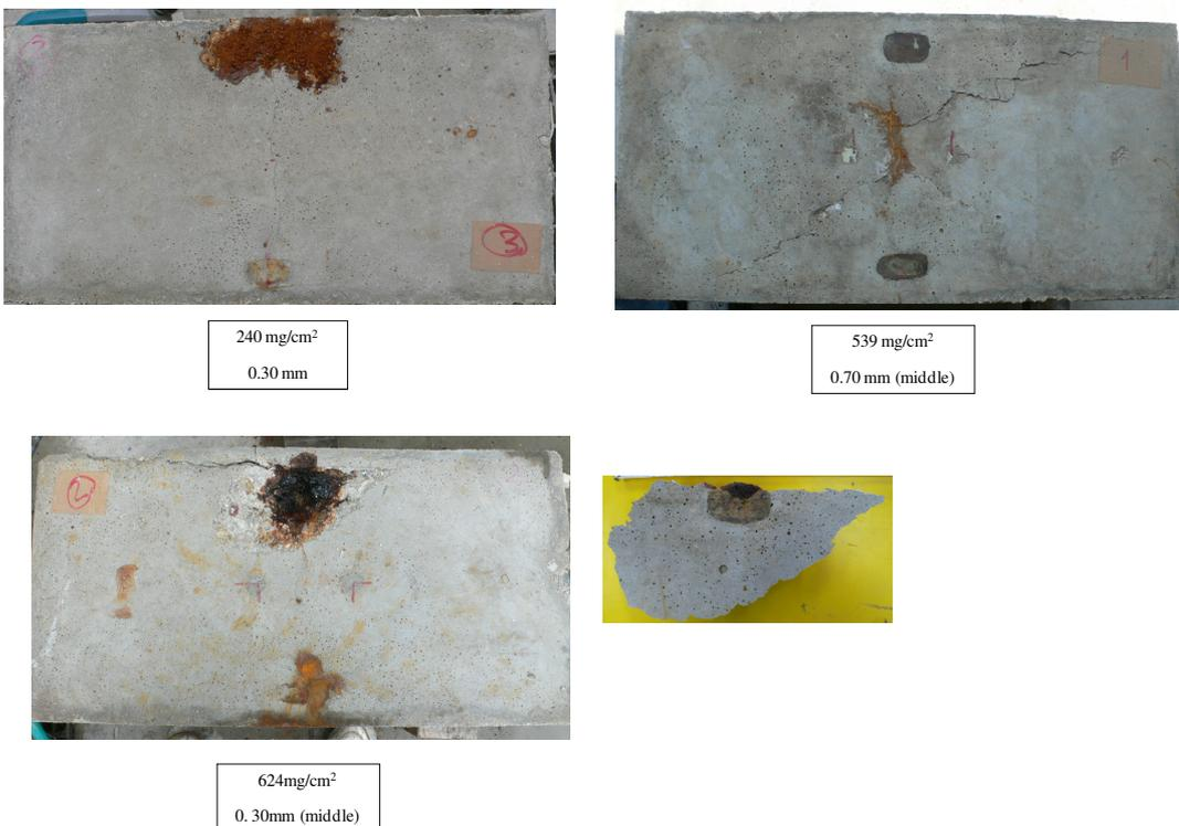
Figure B.37. Surface crack pattern of 600\*400-C30
