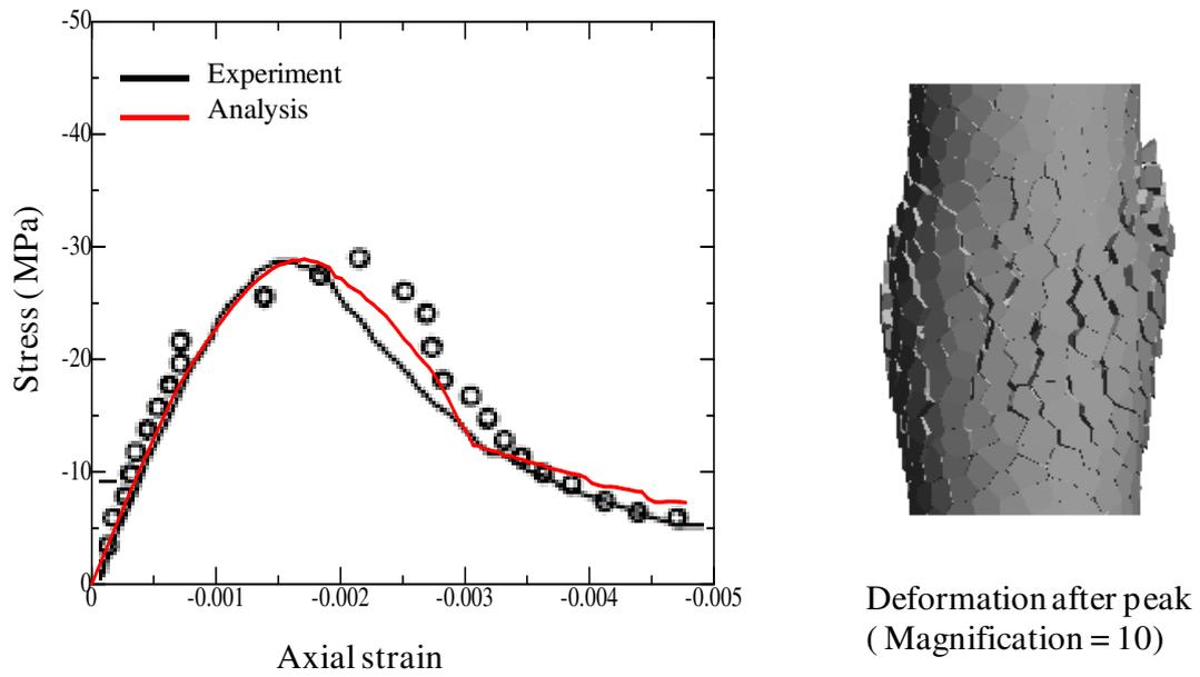
**Figure A.9.** Analytical results of cylinder compression specimen
