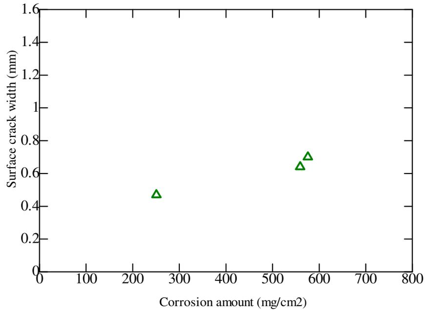
Figure B.16. Surface crack width propagation of 150\*150-D10
