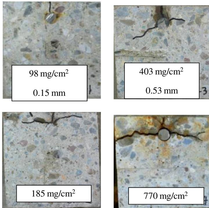
**Figure B.10.** Internal crack patterns of 150\*150-C15
