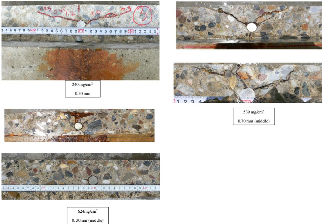
**Figure B.38.** Internal crack pattern of 600\*400-C30
