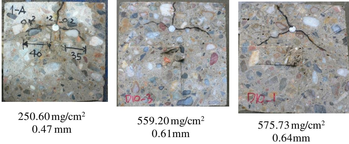
**Figure B.18.** Internal crack patterns of 150\*150-D10
