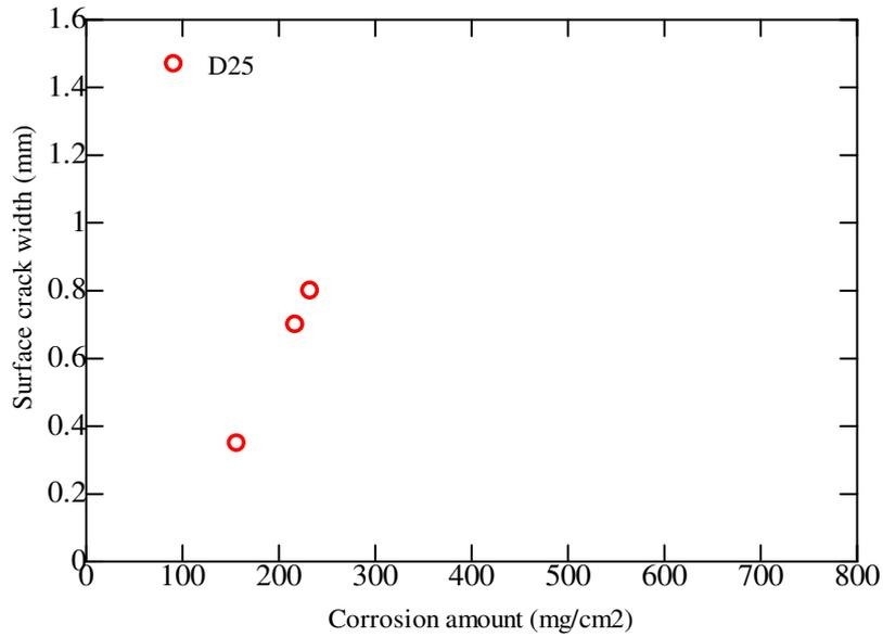
Figure B.20. Surface crack width propagation of 150\*150-D25
