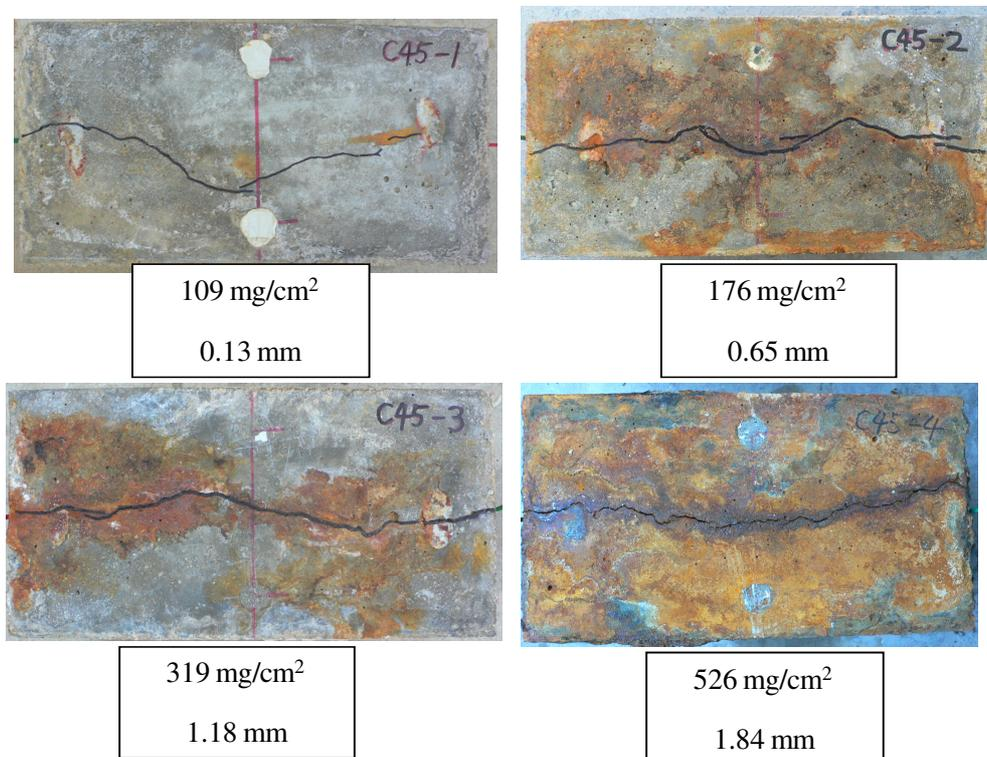
Figure B.13. Surface crack patterns of 150\*150-C45
