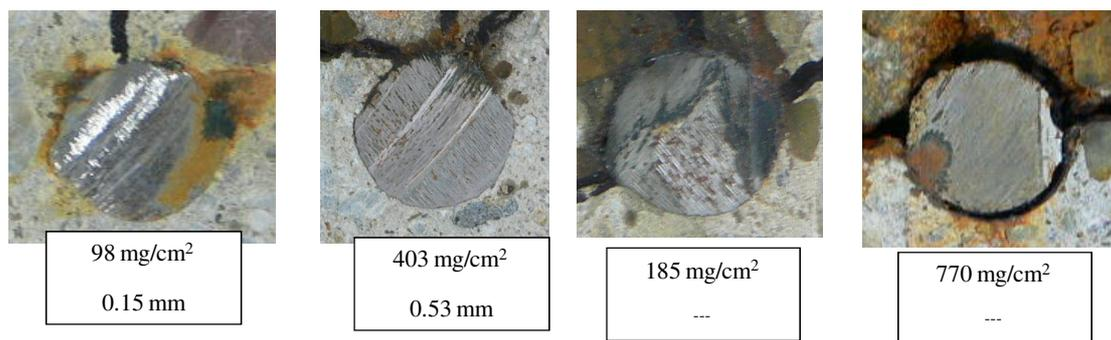
**Figure B.11.** Actual rebar corroded sectional pattern of 150\*150-C15
