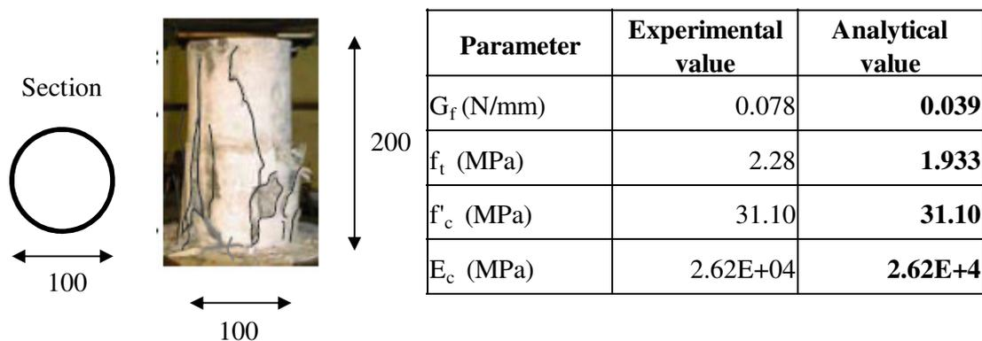
**Figure A.7.** Set-up of cylinder compression test
