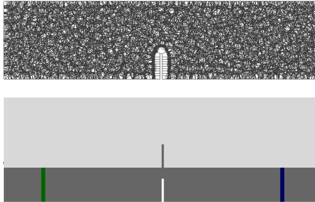
**Figure A.5.** Meshing of pre-cracked 3- point bending test
