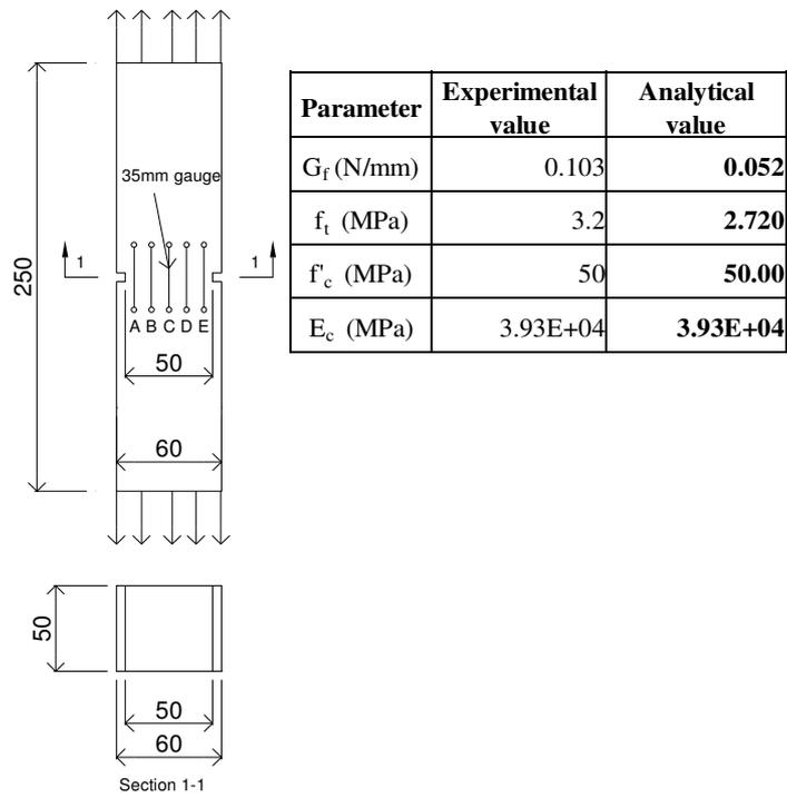
**Figure A.1.** Outline of "direct" tension test
