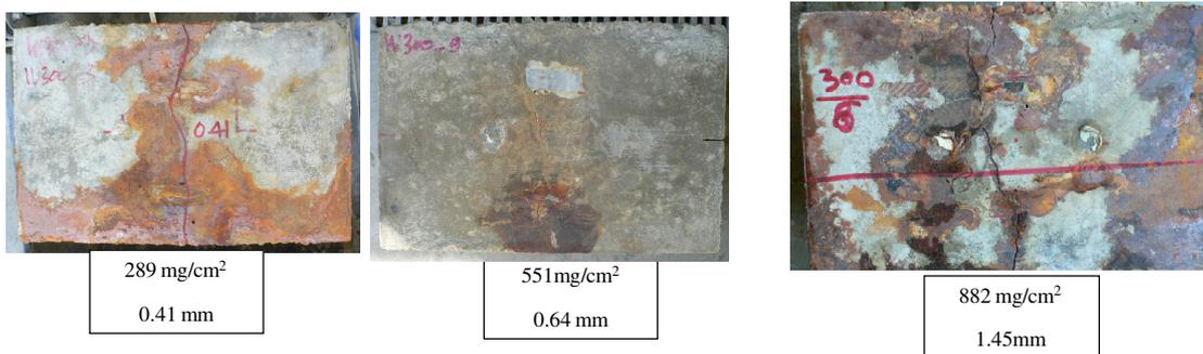
Figure B.25. Surface crack patterns of 300\*150-C30
