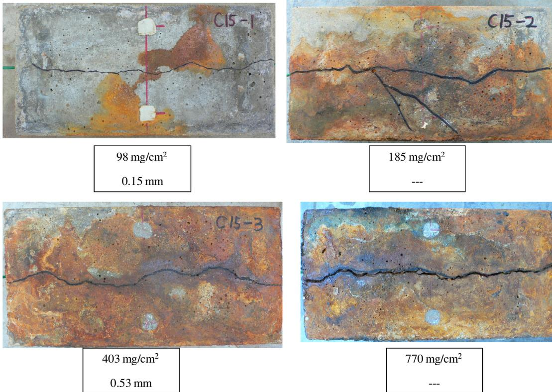
**Figure B.9.** Surface crack patterns of 150\*150-C15
