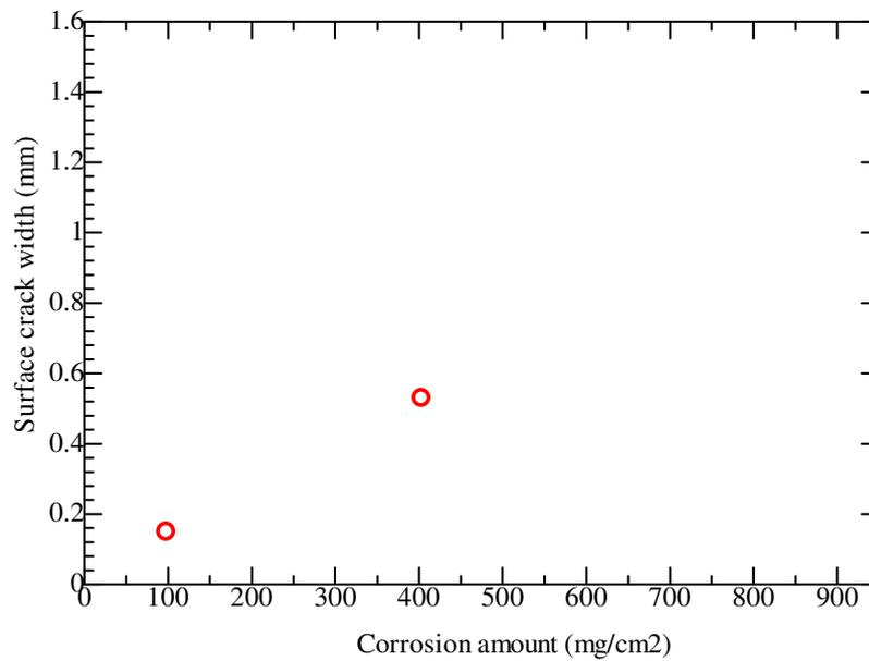
**Figure B.8.** Surface crack width propagation of 150\*150-C15
