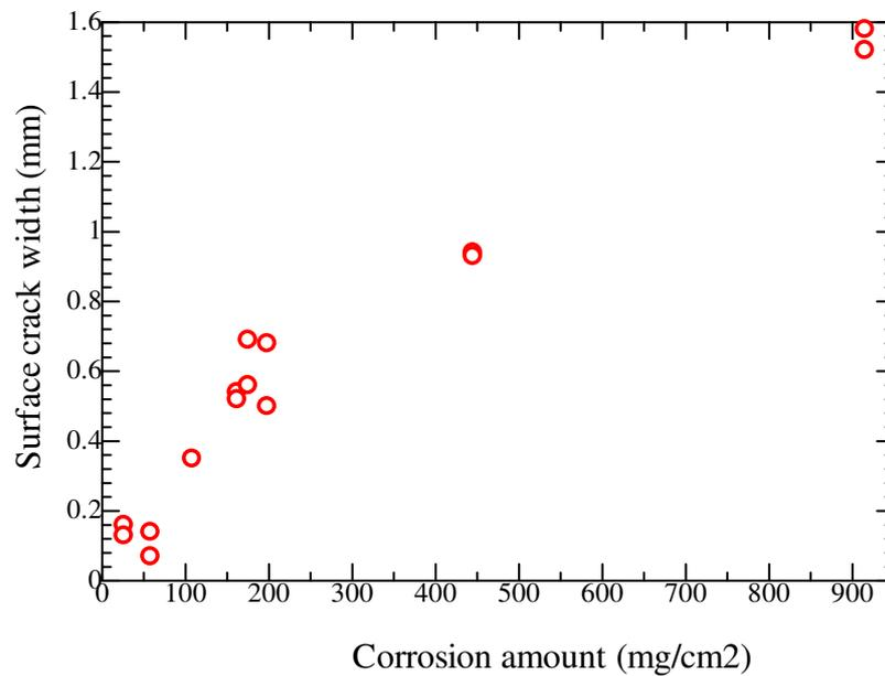
**Figure B.1.** Surface crack width propagation of 150\*150-C30
