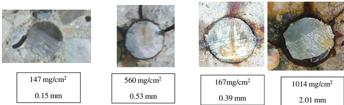
**Figure B.35.** Actual rebar corroded sectional pattern of 400\*400-C30
