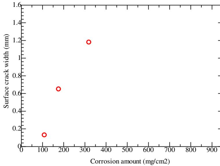
Figure B.12. Surface crack width propagation of 150\*150-C45
