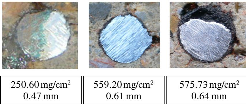
**Figure B.19.** Actual rebar corroded sectional pattern of 150\*150-D10
