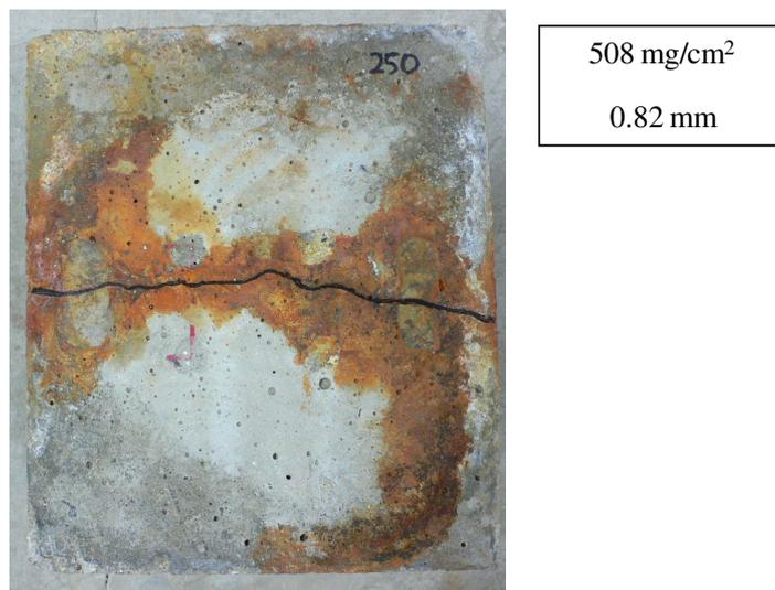
**Figure B.29.** Surface crack pattern of 250\*250-C30
