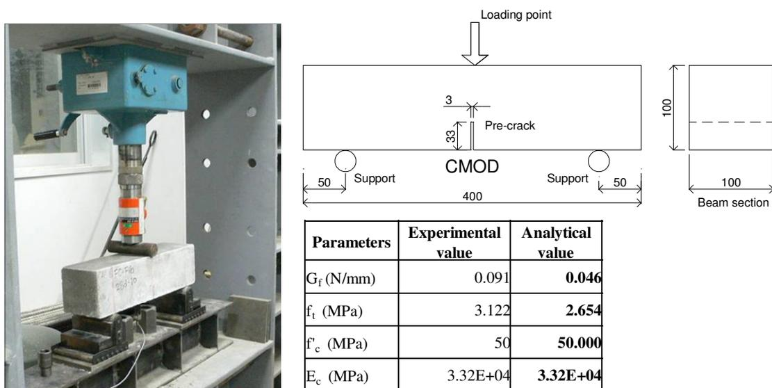
**Figure A.4.** Set-up of pre-cracked three point bending specimen
