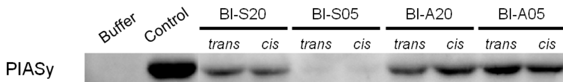
Figure 3-17. Effect of trans - and cis -azobenzene isomerized by UV irradiation on the RNAi activity. For the trans \rightarrow cis isomerization, a UV-D36C filter (Asahi Tech. Co.) was used, and UV light ( \lambda = 300\text{-}400\text{ nm} ; 5.3\text{ mW cm}^{-2} ) was irradiated to the solution of the duplex at 60^\circ\text{C} for 3 min. Photo-isomerization was carried out before transfection.
