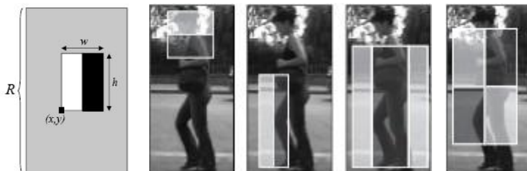
Fig. 3.7 Examples of filters that give high response in regions containing pedestrians.
