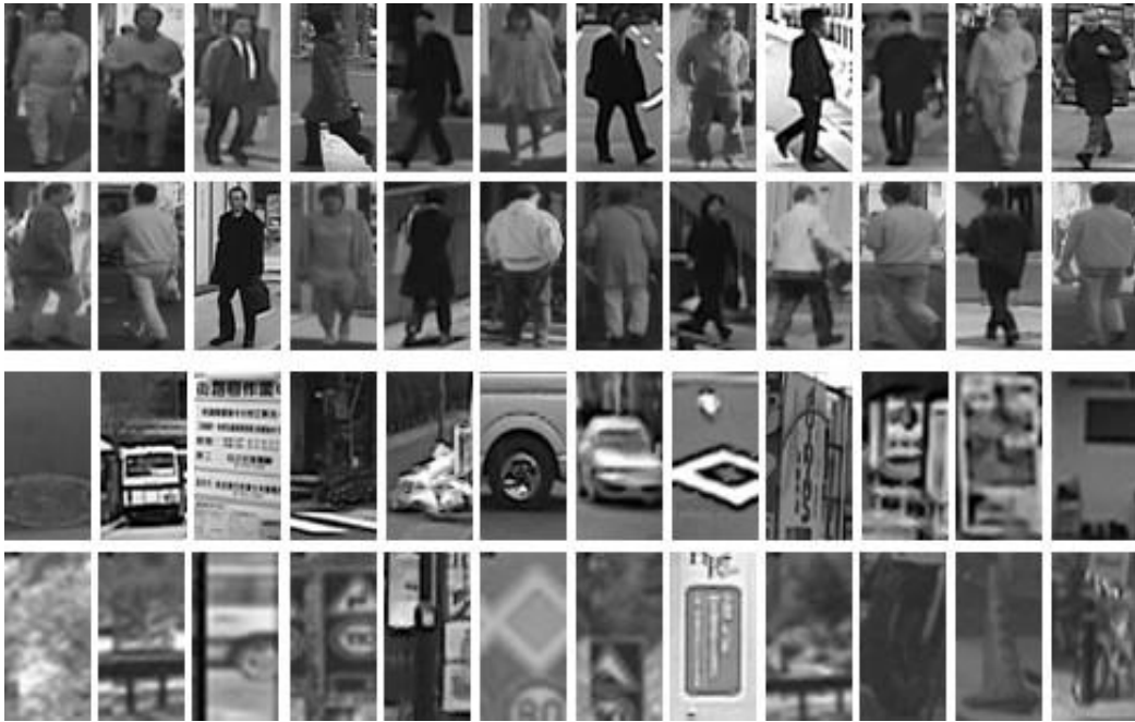
Fig. 3.10 Positive training samples (top two rows) and negative training samples (bottom two rows)
