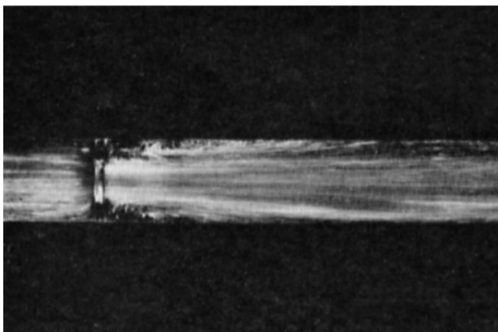
FIG. 6. Steep stenosis. The inner diameter of the stenosis is 5.1 mm. 300 ml/min. Eddy is in the poststenotic marginal area. Stagnation is observed just distal to the stenosis proximal to the eddy currents.
