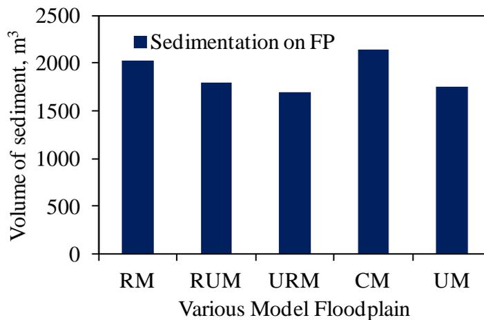
**Fig. 6.14** Sediment deposition comparisons on floodplain of different typical model flood plains.
