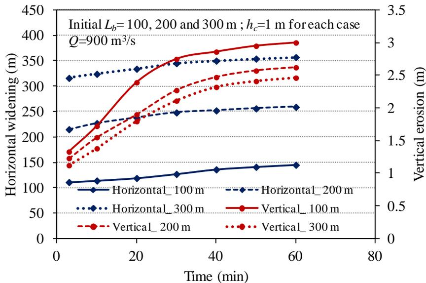
**Fig. 2.25** Relationships between the horizontal widening and vertical erosion of the levee with time for different initial breach length in the levee
