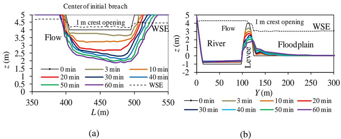
**Fig. 2.10** Evolution process of levee reach with time: (a) temporal growth of breaching section (front view at  $y=115$  m); (b) temporal loss of levee cross section (side view at  $L=475$  m).
