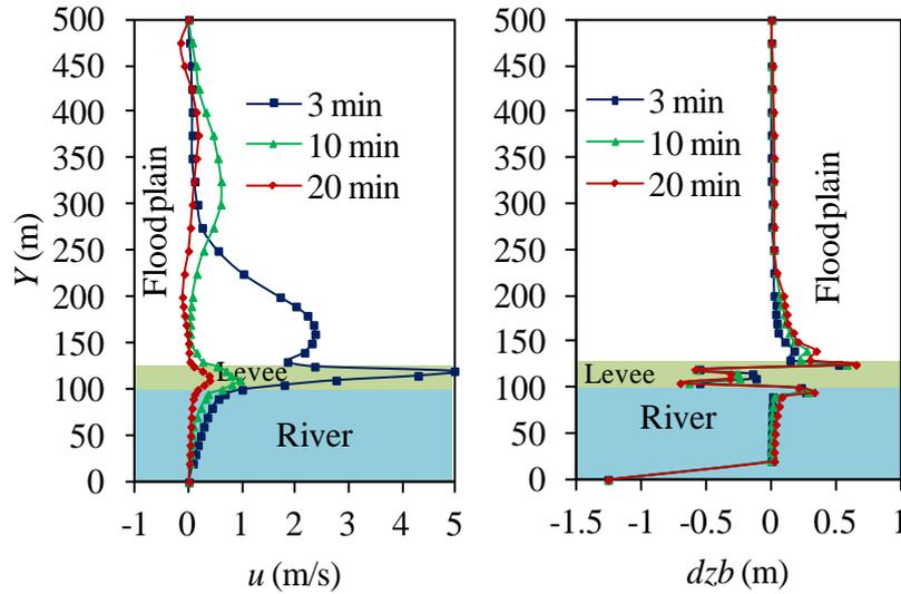
**Fig. 2.14** Transverse distribution of velocity ( $u$ ) and sedimentation ( $dzb$ ) profile at  $L=475$  m on breach with time where  $h_c=4$  m from floodplain.
