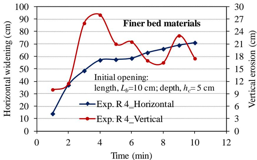
**Fig. 3.11** Relationships between horizontal widening and vertical erosion of the levee with time for experimental Run 4
