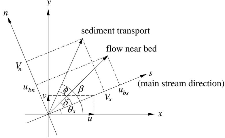
**Fig. 2.4** Angles of flow and sediment transport direction
