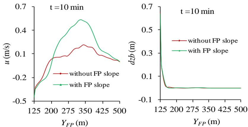
**Fig. 2.15** Comparison of transverse velocity and sedimentation profile in the floodplain at  $L=450$  m on breach considering with and without floodplain slope where  $h_c=4$  m from Floodplain
