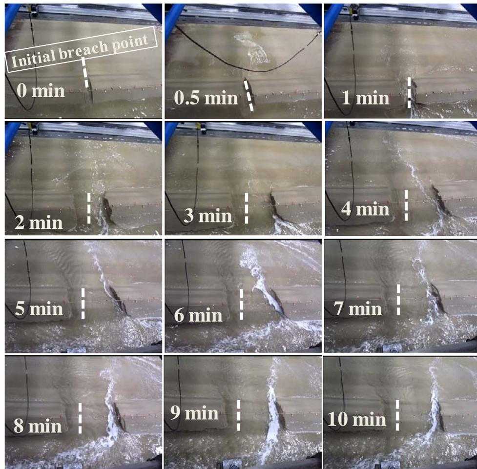
**Photo 3.6** Levee breaching process and bed topographic changes with time due to overflow levee breach (Run 6).
