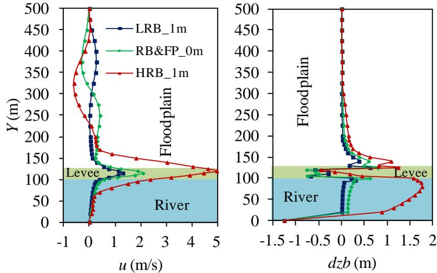
**Fig. 2.31** Transverse distribution of velocity ( $u$ ) and sedimentation ( $dzb$ ) profile after 15 minutes at  $L=475$  m on breach with various river bed levels where  $h_c=4$  m from floodplain
