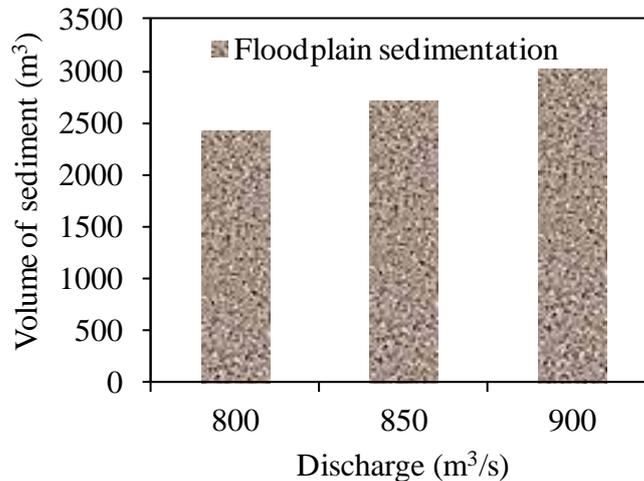
**Fig. 2.21** Comparisons of sedimentation on floodplain for different inflow discharges
