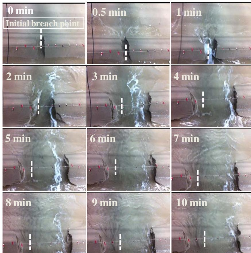
**Photo 3.4** Levee breaching process and bed topographic changes with time due to overflow levee breach (Run 5).
