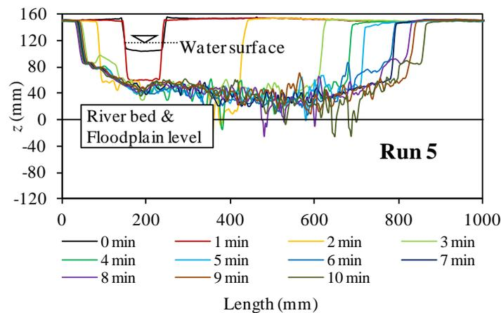
**Fig. 3.13** Breach evolution processes with time along the longitudinal direction of the river (Run 5).
