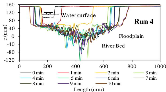
**Fig. 3.10** Breach evolution processes with time along the longitudinal direction of the river (Run 4).
