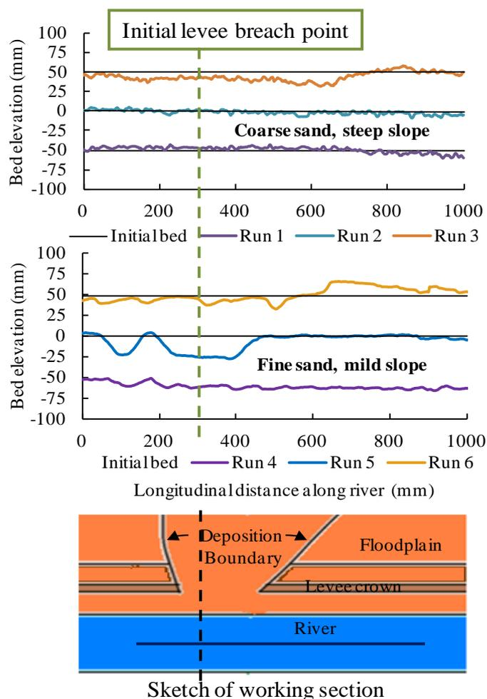
**Fig. 3.24** Comparisons of the river bed variations ( $t=10$  min) at different river bed conditions (Run 1 to 6).
