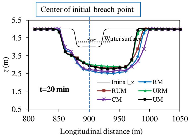
**Fig. 6.12** Longitudinal breach length of the levee (top) along the river for different model flood plains.
