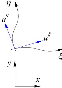
**Fig. 2.1** Moving boundary-fitted coordinate system with contra variant components of velocity
