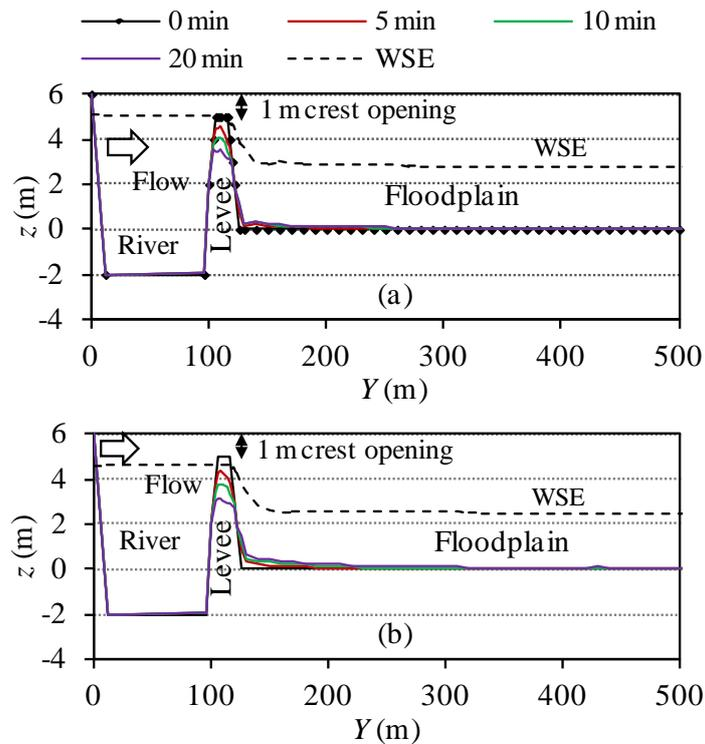
**Fig. 5.5 (ii)** Comparison of temporal loss of levee cross section at  $L=920$  m with time: (a) Bangladesh Model and (b) Japanese Model.
