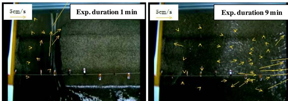
**Fig.3.15** Flow velocity vector analyzed by LSPIV technique (Run3)
