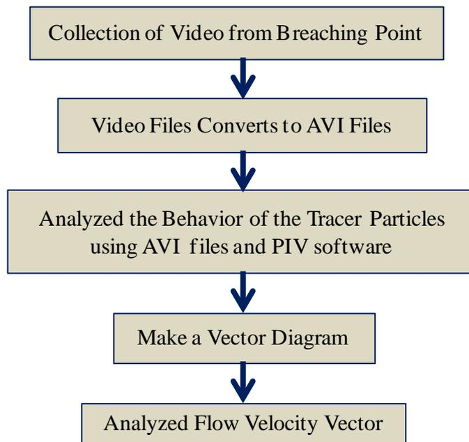
**Fig. 3.7** A flow-chart to analyzed velocity vector using PIV software.
