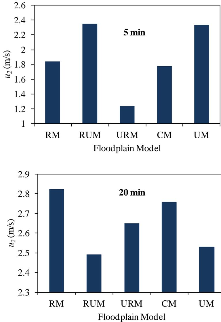
**Fig. 6.11** Transverse velocity profile at the center of an initial breach point ( $L=900$  m) of the levee for different model flood plains.
