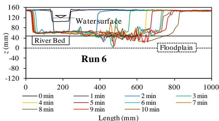
**Fig. 3.17** Breach evolution processes with time along the longitudinal direction of the river (Run 6).
