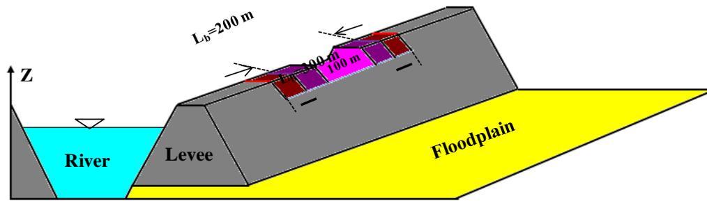
**Fig. 2.22** Defining sketch of initial breach opening of the levee
