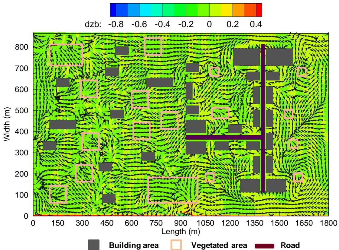
**Fig. 6.5** Flow pattern and sedimentation in the floodplain after the levee breach for Rural-Urban Model [RUM] flood plains.
