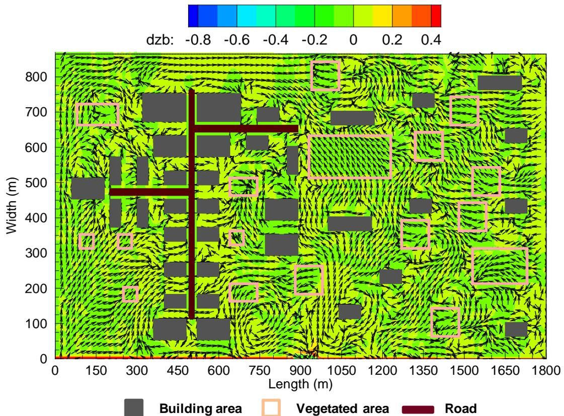
**Fig. 6.6** Flow pattern and sedimentation in the floodplain after the levee breach for Urban-Rural Model [URM] flood plains.
