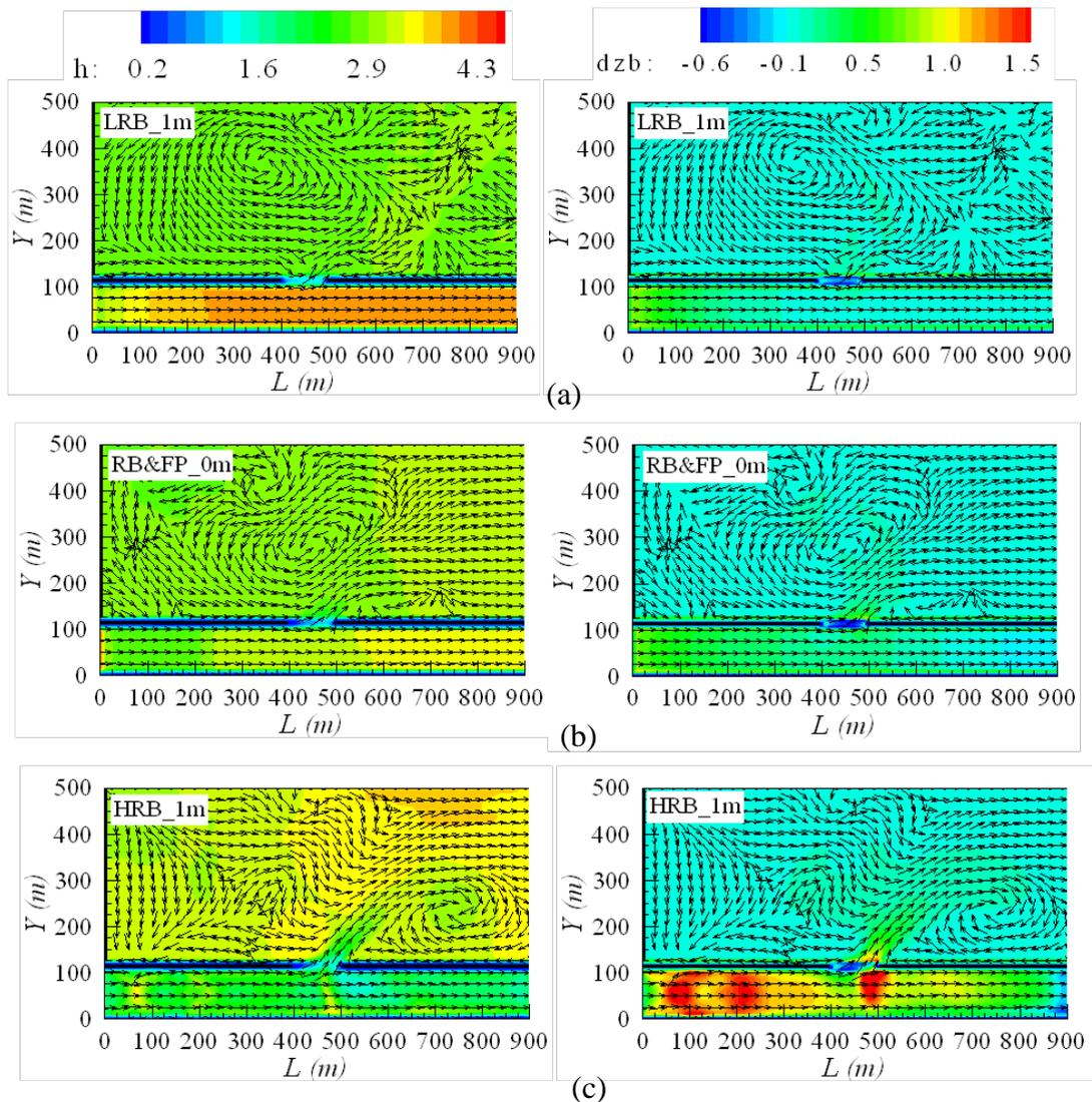
**Fig. 2.30** Spatial characteristics of flow and morphological changes at levee breach with various river bed level changes as compared with floodplain level ( $t=15$  min): (a) LRB\_1 m; (b) RB and FP at same level; and (c) HRB\_1 m, where  $h_c=4$  m from floodplain; contours indicate the water depth ( $h$ ) and deviation of bed elevation ( $dzb$ ).
