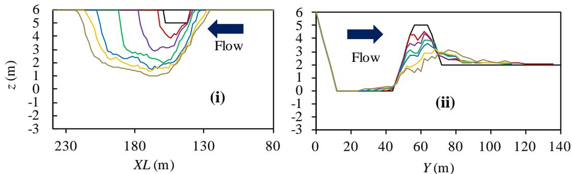
(b) RIC-Nays Model results: (i) Growth of breaching section at  $y = 62$  m (front view)
