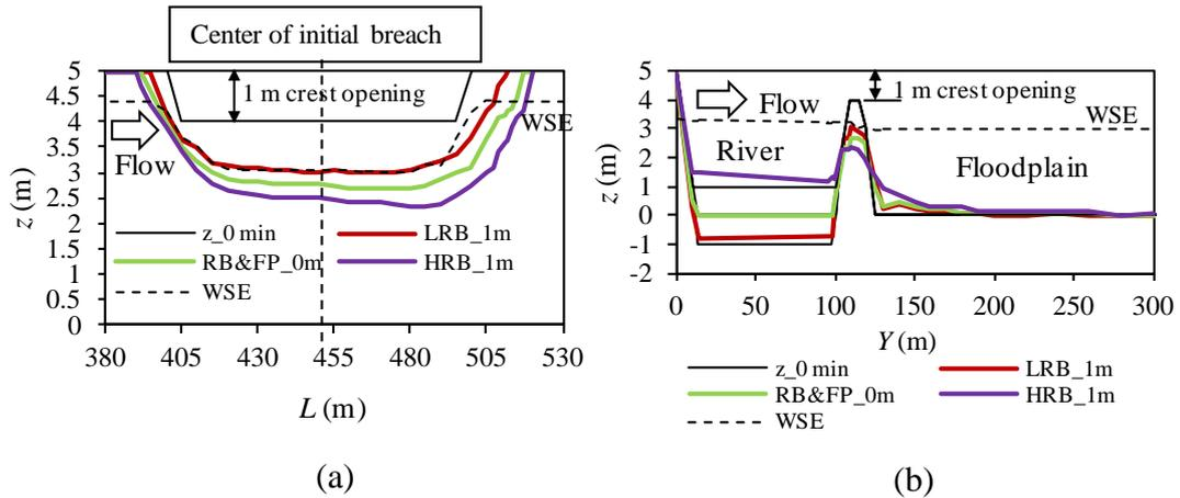
**Fig. 2.32** Evolution process of levee reach due to different river bed levels: (a) temporal growth of breaching section (front view at  $y=115$  m); (b) temporal loss of levee cross section (side view at  $L=475$  m).
