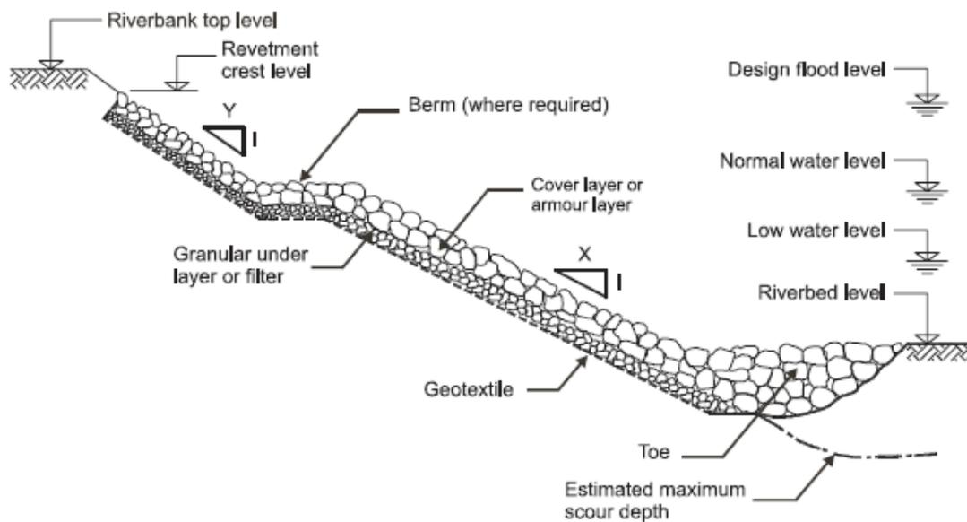
**Fig. A. 9** Typical layout of revetment works
