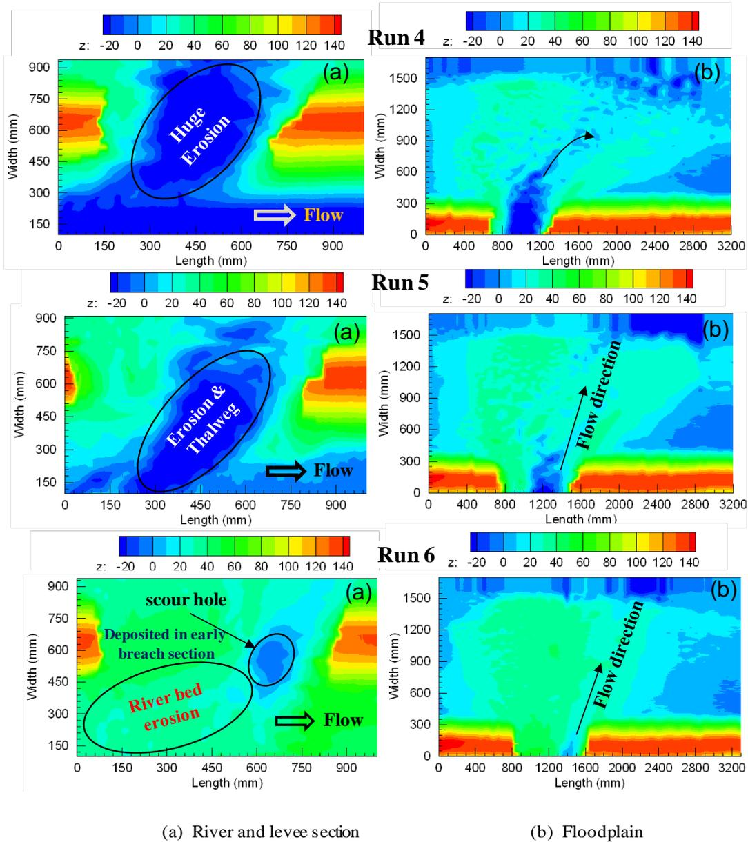
**Fig. 3.22** Comparisons of final bed topographic changes in the river, levee and floodplain for the Run 4 (top), Run 5 (middle), and Run 6 (below) at same duration ( $t=10$  min).
