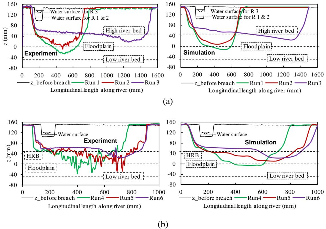
**Fig. 4.8** Comparisons of the final longitudinal lengths of breach along the river for experiments and simulation ( $t=10$  minutes): (a) Runs 1 to 3; and (b) Runs 4 to 6.
