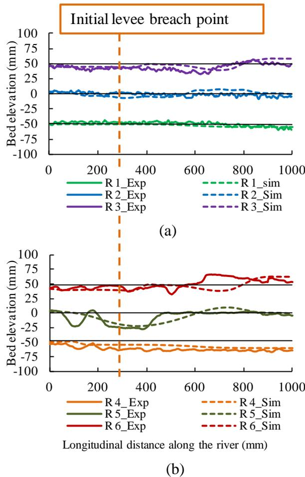
**Fig. 4.9** Comparisons of river bed variations along the river for experiments and simulation: (a) Runs 1 to 3; and (b) Runs 4 to 6.
