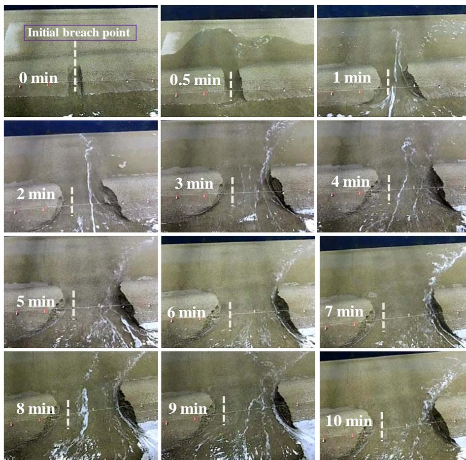
**Photo 3.1** Levee breaching process and bed topographic changes with time due to overflow levee breach (Run 1).
