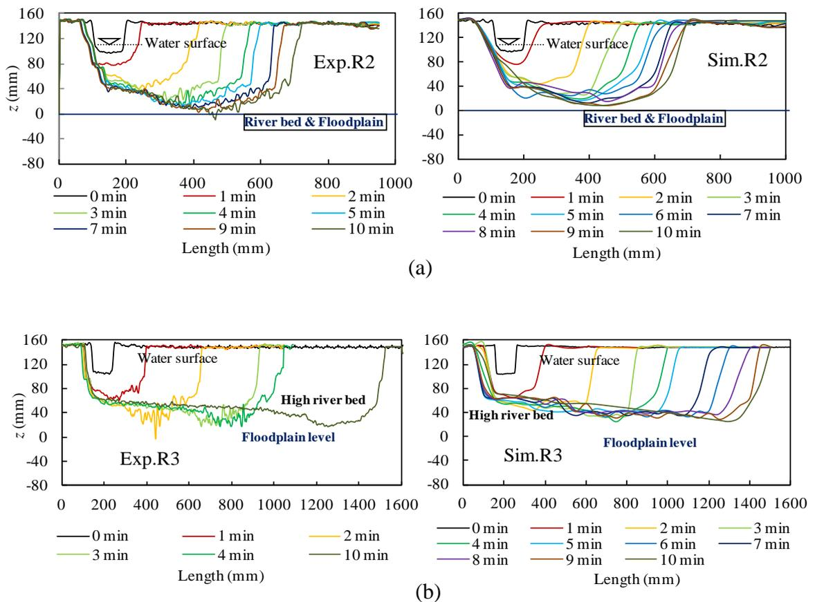
**Fig. 4.4** Longitudinal breach evolution processes of levee with time both in experiment and simulation: (a) Run 2 (Exp.R2, Sim.R2); and (b) Run 3 (Exp.R3, Sim.R3).
