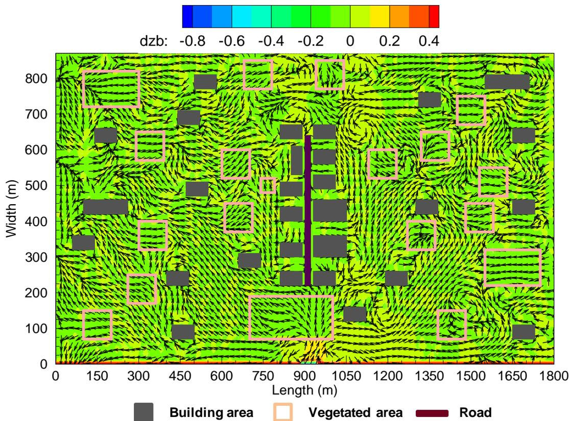
Fig. 6.7 Flow pattern and sedimentation in the floodplain after the levee breach for Combined Model [CM] flood plains.
