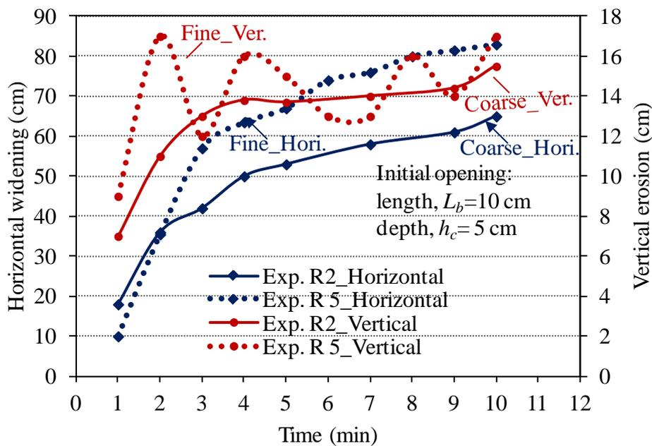
**Fig. 3.14** Relationships between horizontal widening and vertical erosion of the levee with time for experiments: (a) Run 2; (b) Run 5
