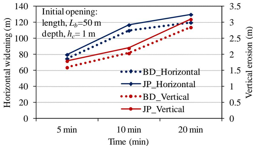
**Fig. 5.6** Relationships between horizontal widening and vertical erosion of the levee with time for Bangladesh (BD) and Japanese (JP) model
