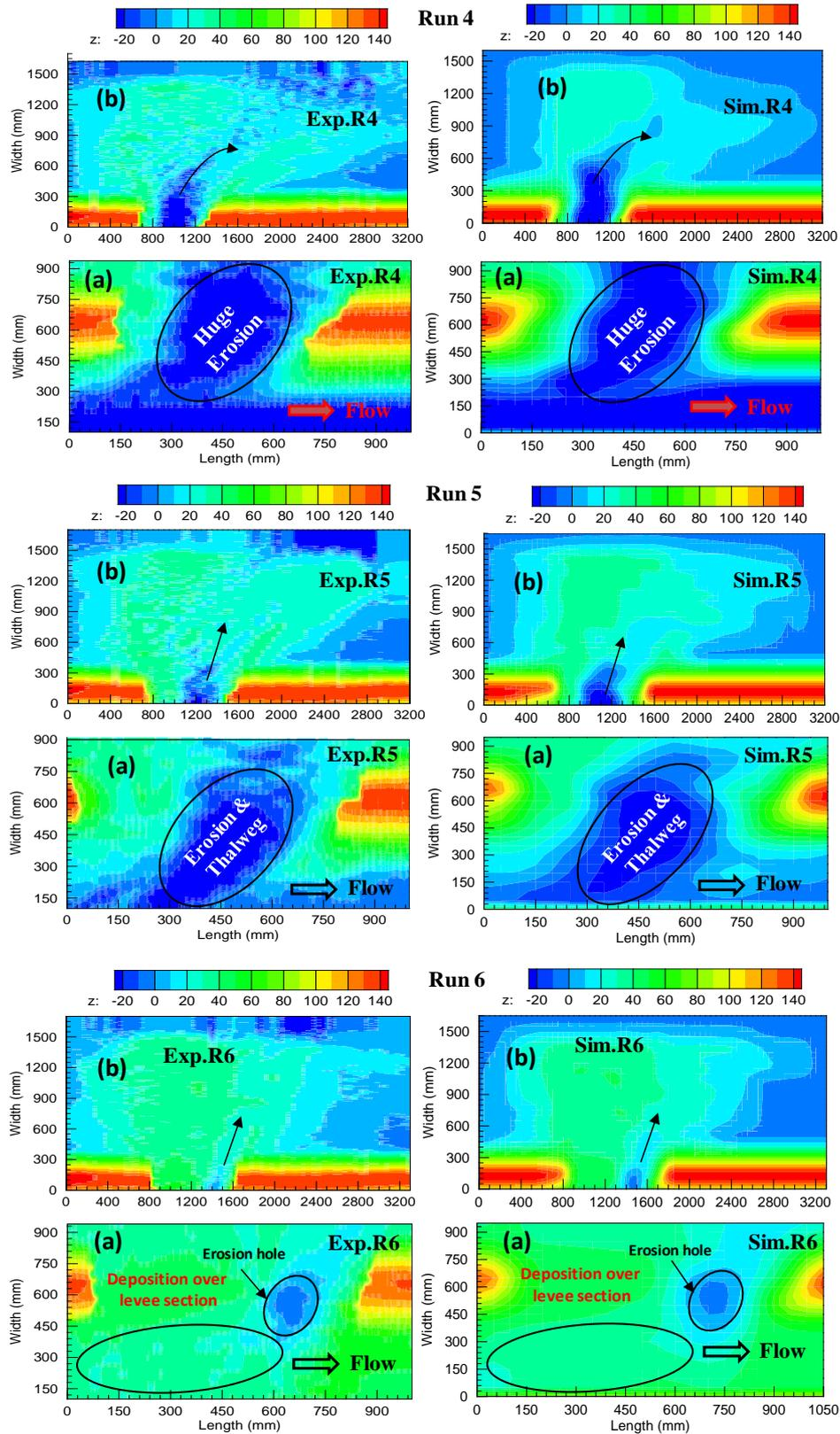
**Fig. 4.5** Experiments (Exp.R4, Exp.R5 and Exp.R6) and simulation (Sim.R4, Sim.R5 and Sim.R6) results of bed topographic changes ( $t=10$  min): (a) River channel and levee section; (b) Floodplain.
