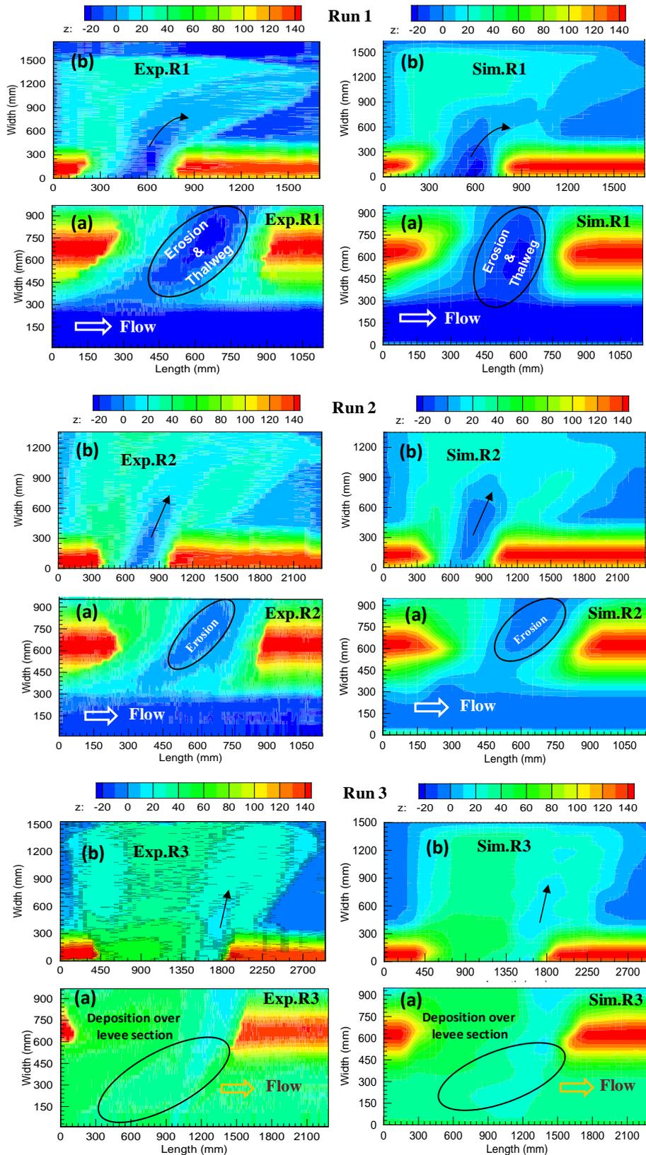
**Fig. 4.3** Experiments (Exp.R1, Exp.R2 and Exp.R3) and simulation (Sim.R1, Sim.R2 and Sim.R3) results of bed topographic changes ( $t=10$  min): (a) River channel and levee section; (b) Floodplain.
