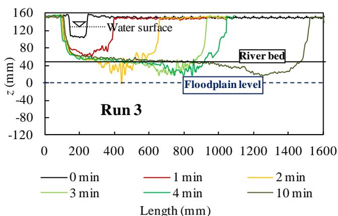
**Fig. 3.16** Breach evolution processes with time along the longitudinal direction of the river (Run 3).
