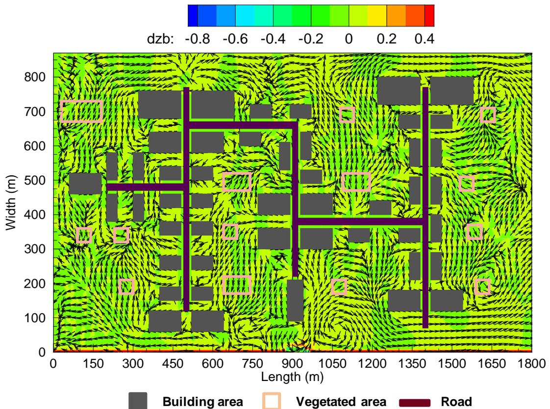
**Fig. 6.8** Flow pattern and sedimentation in the floodplain after the levee breach for Urban Model [UM] flood plains.
