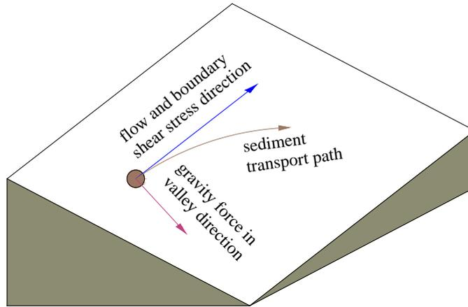
**Fig. 2.2** Gravity effect on sediment particles
