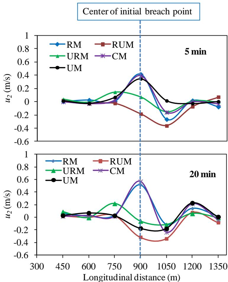
**Fig. 6.10** Transverse velocity profile in the floodplain ( $y=45$  m) along the levee for different model flood plains.
