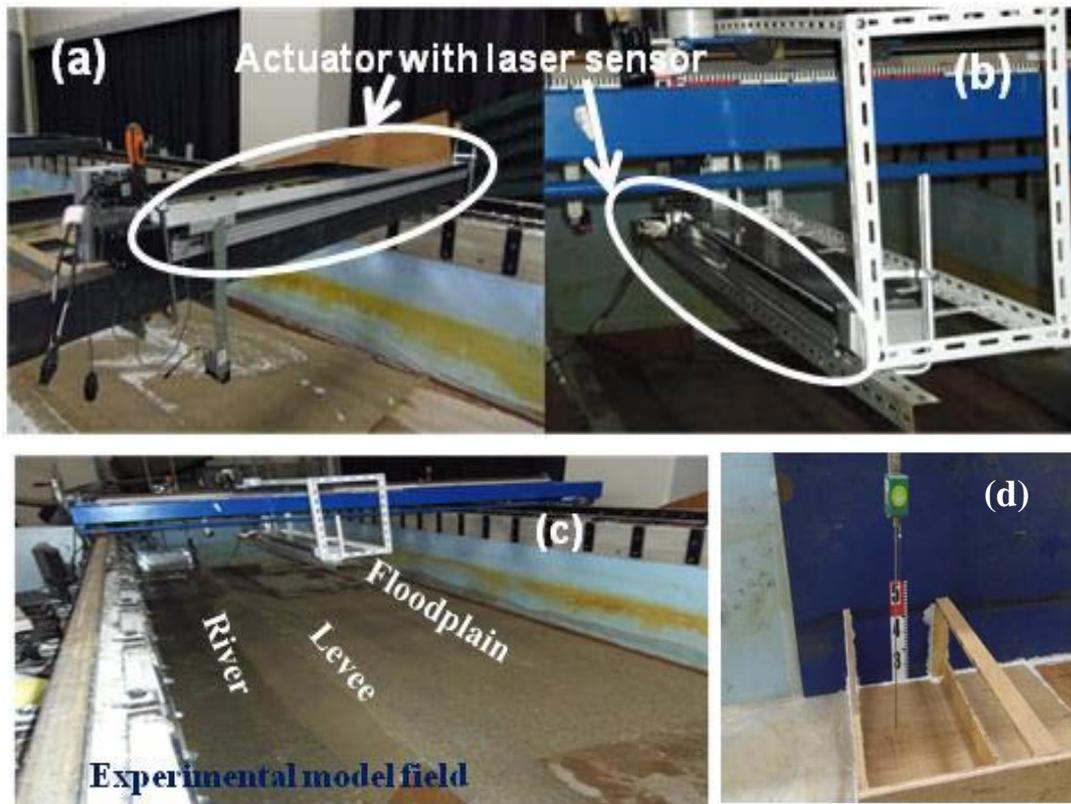
**Fig. 3.3** Electronic actuator with computer aided laser sensor: (a) lateral and (b) longitudinal direction; (c) experimental model field; (d) a wave meter setting.
