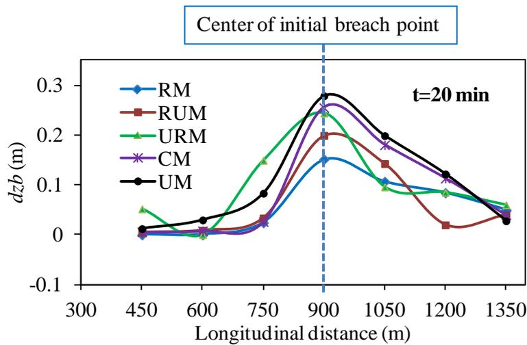
**Fig. 6.13** Comparisons of depth of deposition on the floodplain ( $y=45$  m) along the levee for different model flood plains.
