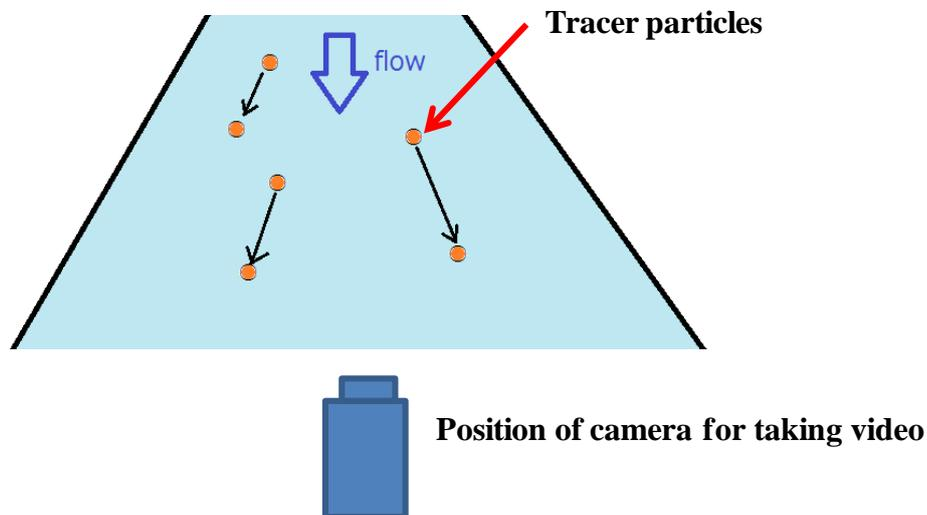
**Fig. 3.6** Schematics diagram of the collection of a video file.
