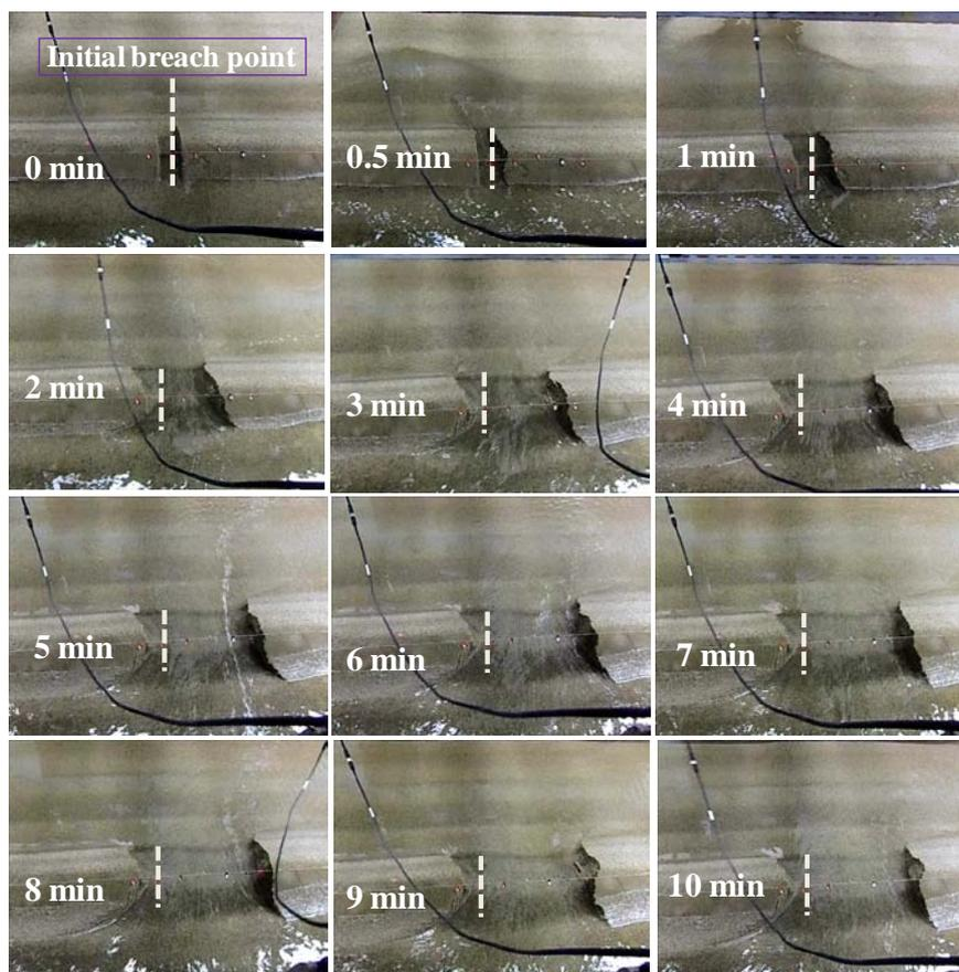
**Photo 3.3** Levee breaching process and bed topographic changes with time due to overflow levee breach (Run 2).
