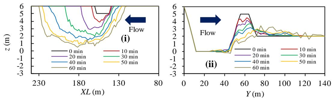
(a) NHSED2D Model results: (i) Growth of breaching section at  $y = 62$  m (front view)
