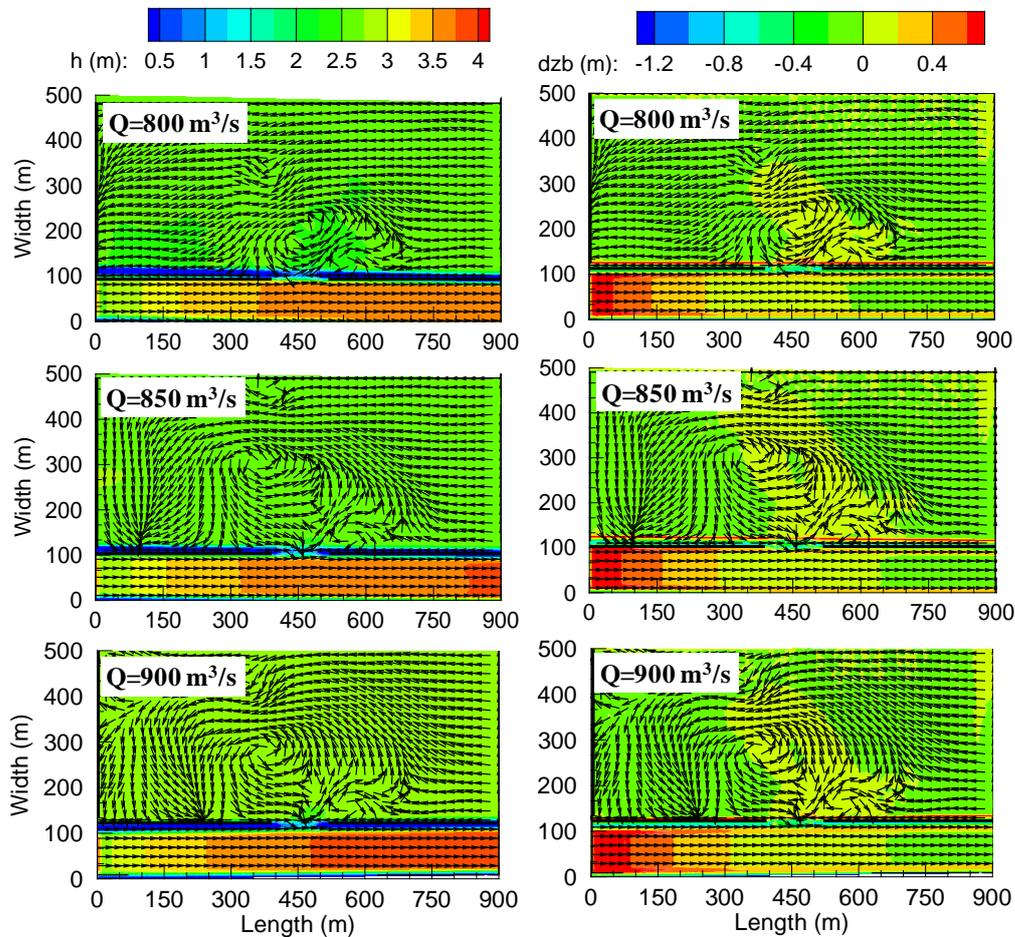
**Fig. 2.19** Simulated flow field in the vicinity of the river, breach levee and floodplain where  $h_c=4$  m from floodplain; contours indicate the water depth ( $h$ ) and deviation of bed elevation ( $dzb$ ) at 800, 850 and 900  $\text{m}^3/\text{s}$  discharges (top to bottom), respectively.
