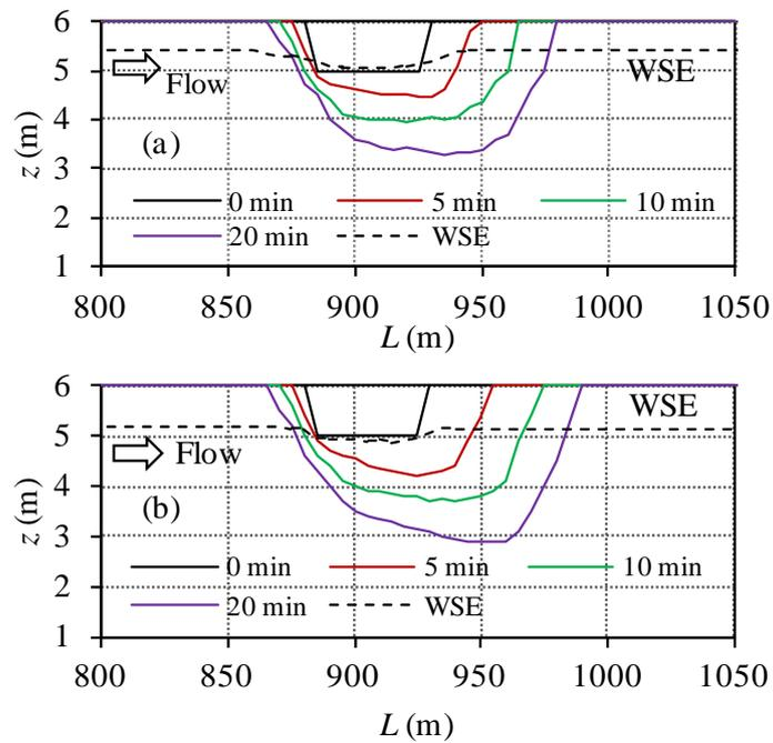
**Fig. 5.5 (i)** Comparison of temporal growth of breaching section at  $y=115$  m with time: (a) Bangladesh Model and (b) Japanese Model.
