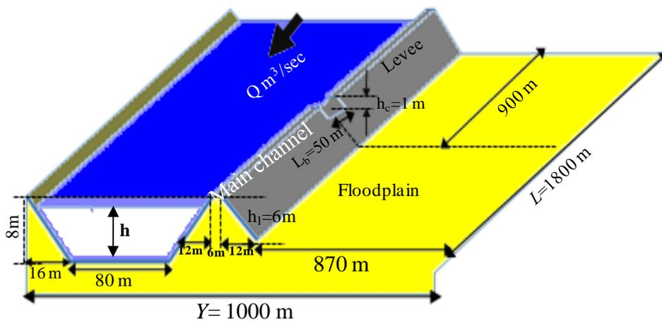
**Fig. 5.1** Simulated model area showing river channel, breach levee and floodplain.
