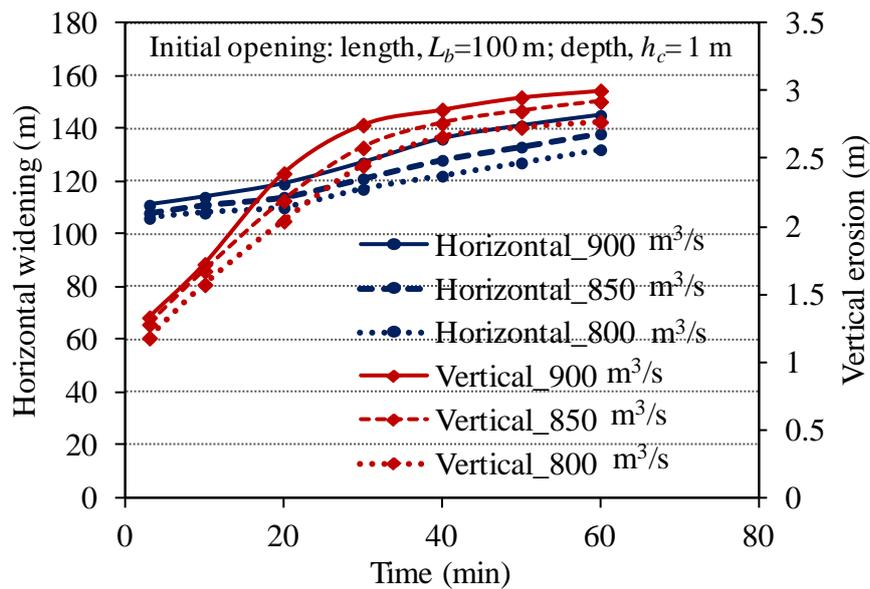
**Fig. 2.18** Relationships between horizontal widening and vertical erosion of the levee with time for different inflow discharges.
