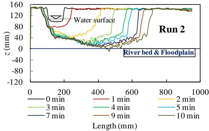
**Fig. 3.12** Breach evolution processes with time along the longitudinal direction of the river (Run 2).
