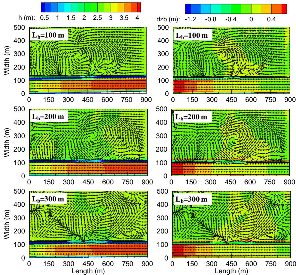
**Fig. 2.26** Simulated flow field in the vicinity of the river, breach levee and floodplain where  $h_c=4 \text{ m}$  from floodplain; contours indicate the water depth ( $h$ ) and deviation of bed elevation ( $dz_b$ ) at 100, 200 and 300 m breach length (top to bottom), respectively.
