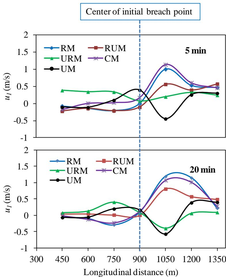
**Fig. 6.9** Longitudinal velocity profile in the floodplain ( $y=45$  m) along the levee for different model flood plains.
