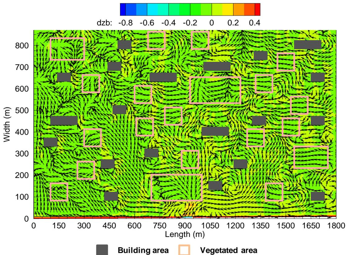
**Fig. 6.4** Flow pattern and sedimentation in the floodplain after the levee breach for Rural Model [RM] flood plains.
