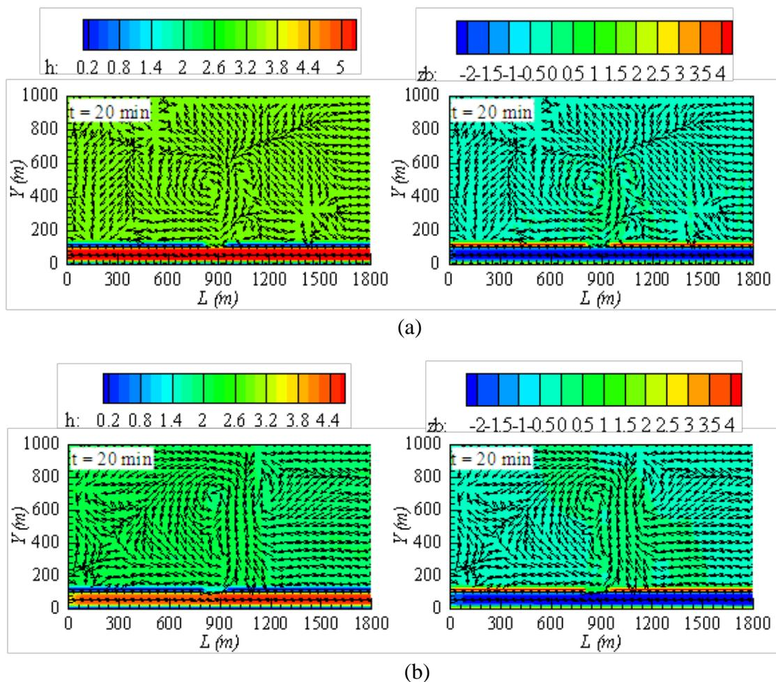
**Fig. 5.3** Characteristics of levee breach flow and morphological changes: (a) Bangladesh Model; and (b) Japanese Model, where  $h_c=5$  m from floodplain; contours indicate the water depth ( $h$ ) and bed elevation ( $z_b$ ).
