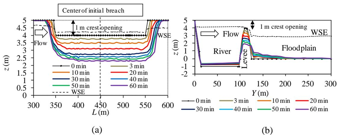
**Fig. 2.23** Evolution process of levee reach with time for  $L_b=200 \text{ m}$ : (a) temporal growth of breaching section (front view at  $y=115 \text{ m}$ ); (b) temporal loss of levee cross section (side view at  $L=475 \text{ m}$ ).
