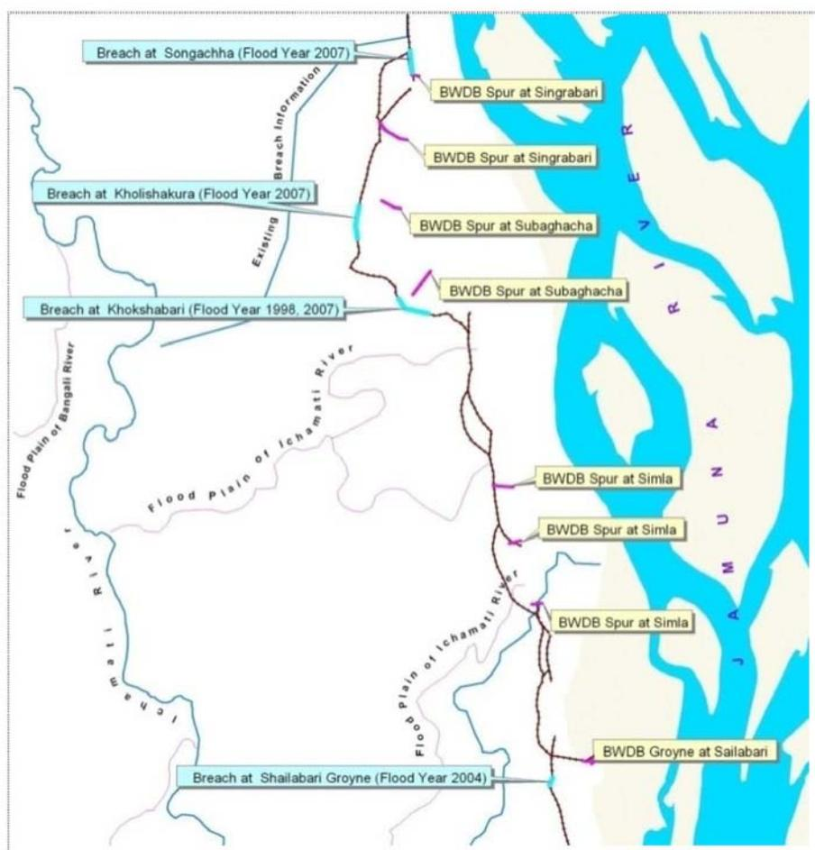
**Fig. A. 5** Breaches at Jamuna River flood protection right bank levee.
