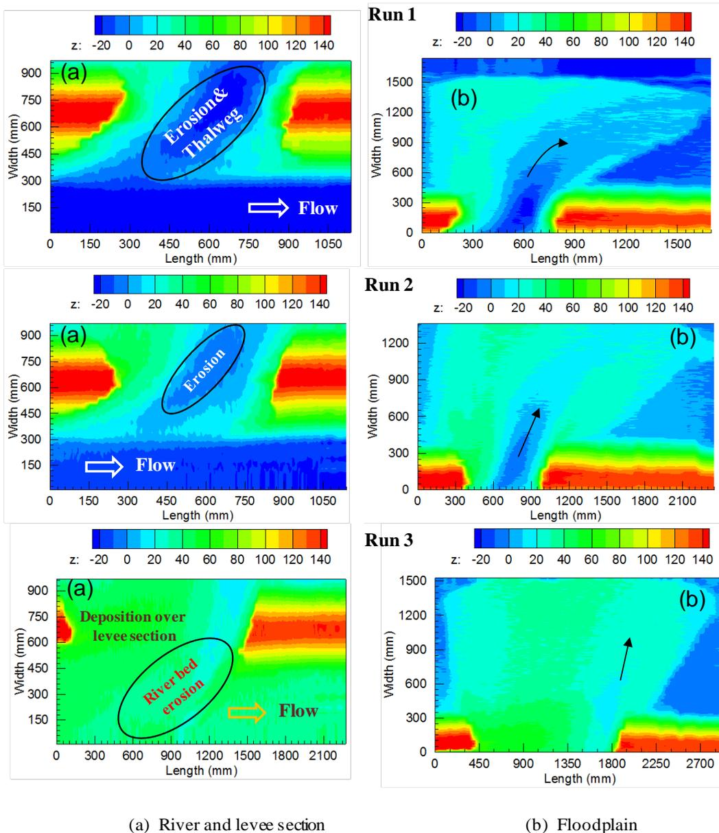
**Fig. 3.20** Comparisons of final bed topographic changes in the river, levee and floodplain for the Run 1 (top), Run 2 (middle), and Run 3 (below) at same duration ( $t=10$  min).
