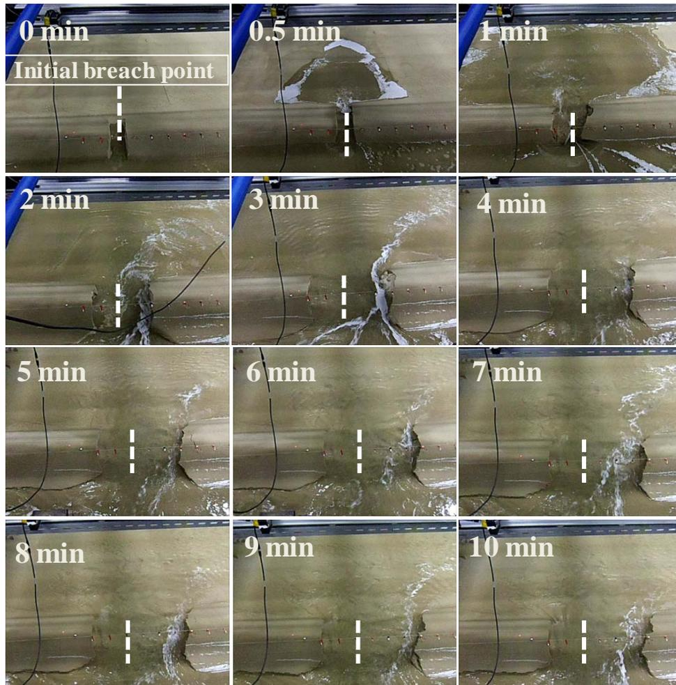
**Photo 3.2** Levee breaching process and bed topographic changes with time due to overflow levee breach (Run 4).
