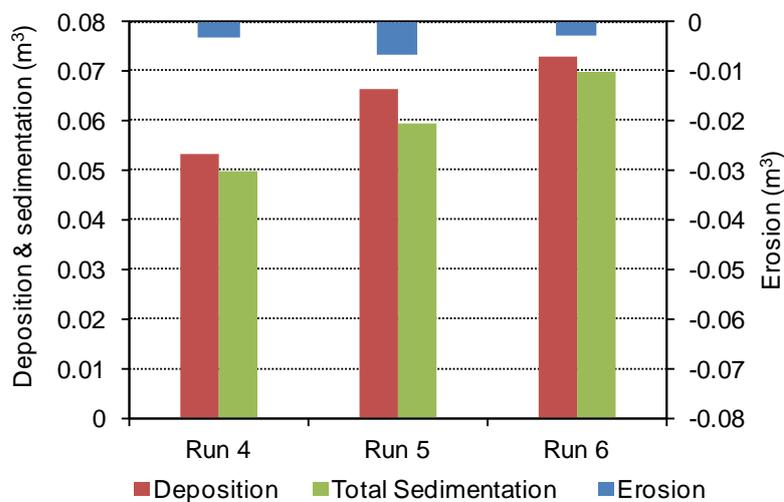
**Fig. 3.23** Comparisons of the volume of the floodplain sedimentation at different relative height of river bed and floodplain (Run 4 to 6).
