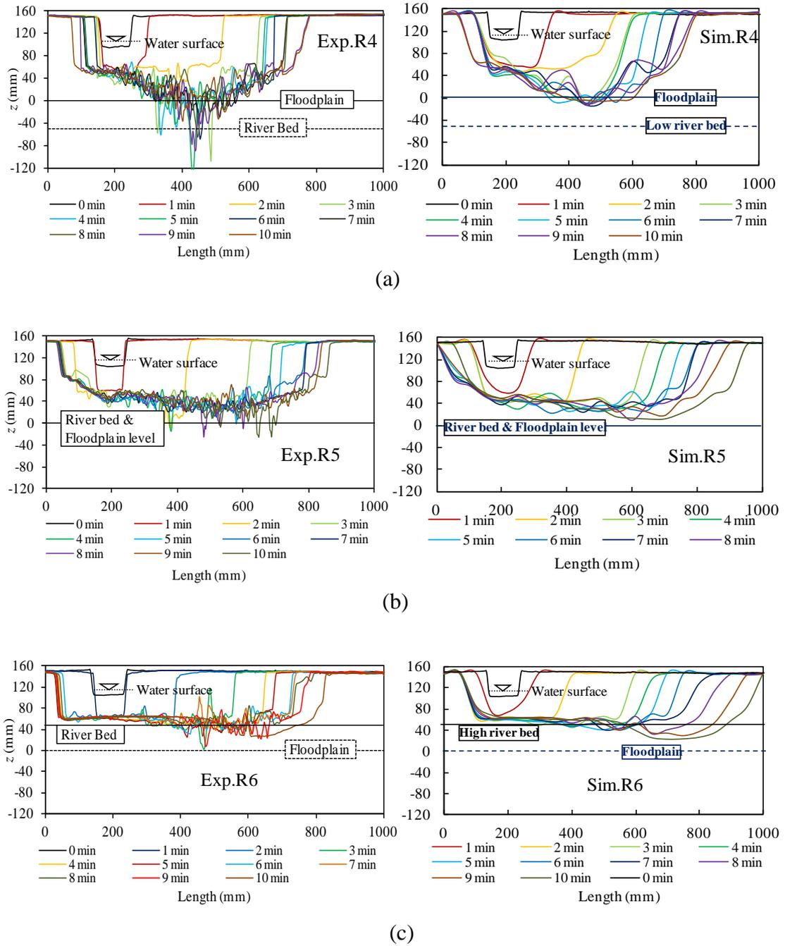
**Fig. 4.6** Longitudinal breach evolution processes of levee with time both in experiment and simulation: (a) Run 4 (Exp.R4 & Sim.R4); (b) Run 5 (Exp.R5 & Sim.R5); and (c) Run 6 (Exp.R6 & Sim.R6).
