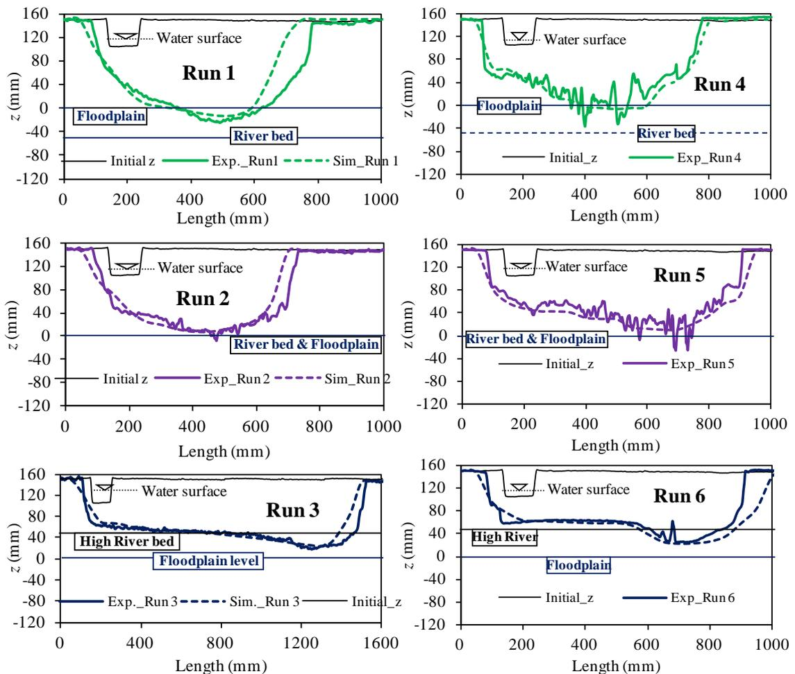
**Fig. 3.25** Comparisons of longitudinal length of breaching ( $t=10$  min) at different height of river bed as compared to floodplain level using experiments and simulation (Run 1 to 6).
