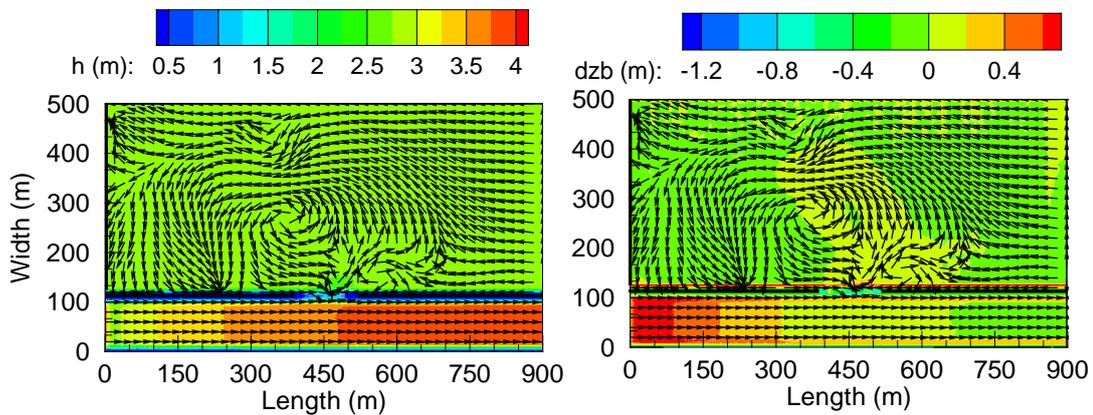
**Fig. 2.12** Spatial characteristics of flow and morphological changes at levee breach ( $t=60$  min); contours indicate the water depth ( $h$ ) and deviation of bed elevation ( $dz_b$ ).
