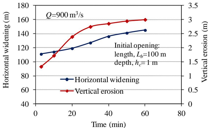
**Fig. 2.11** Relationships between horizontal widening and vertical erosion of the levee with time for inflow discharge of  $900$  m<sup>3</sup>/s.
