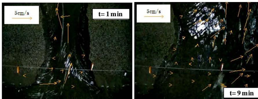
**Fig.3.9** Flow velocity vector analyzed by LSPIV technique (Run1)
