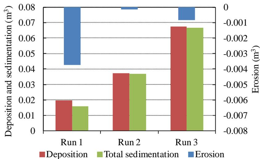
**Fig. 3.21** Comparisons of the volume of the floodplain sedimentation at different relative height of river bed and floodplain (Run 1 to 3).
