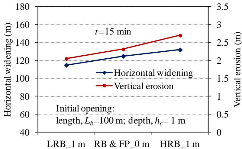
**Fig. 2.33** Relationships between horizontal widening and vertical erosion of the levee with different relative height of river bed to floodplain.
