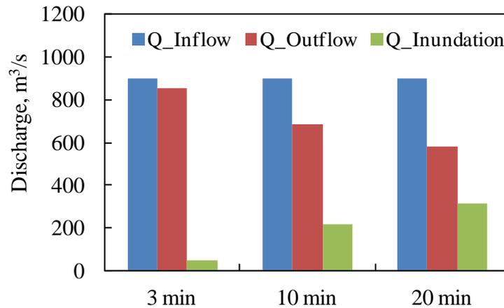
**Fig. 2.13** Discharge into the river and floodplain with time
