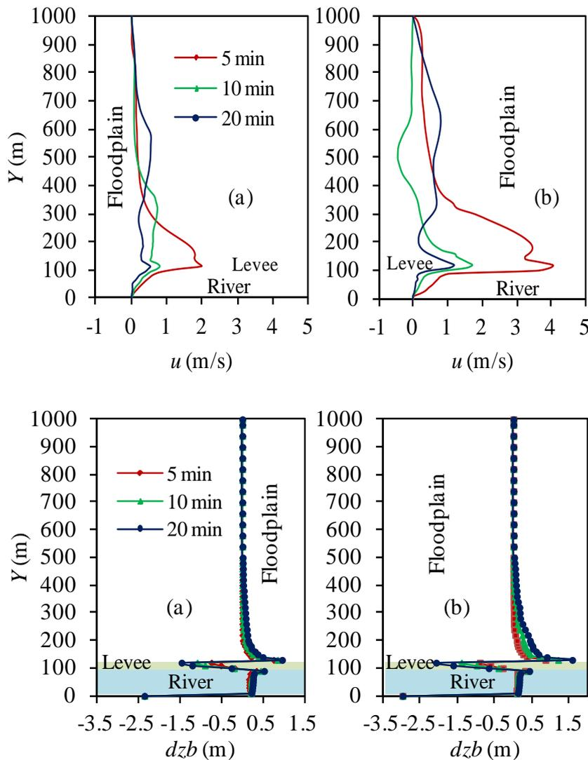
**Fig. 5.4** Comparison of transverse distribution of velocity ( $u$ ) and sedimentation ( $dzb$ ) profile at  $L=920$  m on breach with time: (a) Bangladesh Model and (b) Japanese Model where  $h_c=5$  m from floodplain
