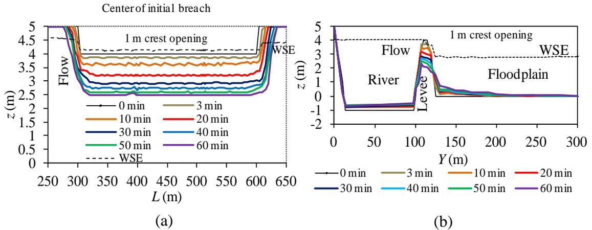
**Fig. 2.24** Evolution process of levee reach with time for  $L_b=300$  m: (a) temporal growth of breaching section (front view at  $y=115$  m); (b) temporal loss of levee cross section (side view at  $L=475$  m).
