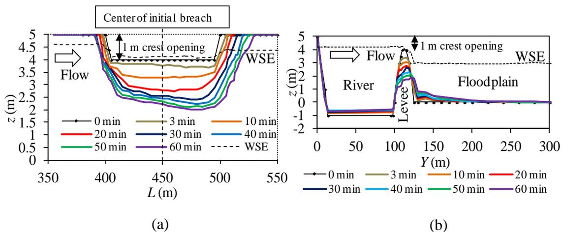
**Fig. 2.17** Evolution process of levee reach with time for  $Q=850 \text{ m}^3/\text{s}$ : (a) temporal growth of breaching section (front view at  $y=115 \text{ m}$ ); (b) temporal loss of levee cross section (side view at  $L=475 \text{ m}$ ).
