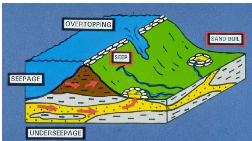
**Fig. A. 13** Schematics diagram of different types of levee failure.
