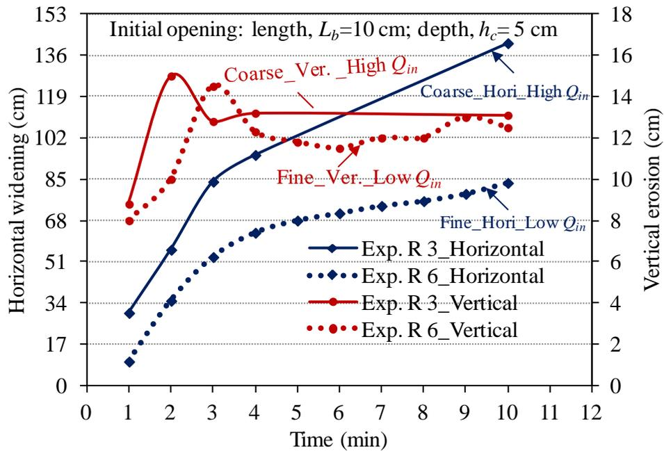
**Fig. 3.18** Relationships between horizontal widening and vertical erosion of the levee with time for experiments: (a) Run 3; (b) Run 6
