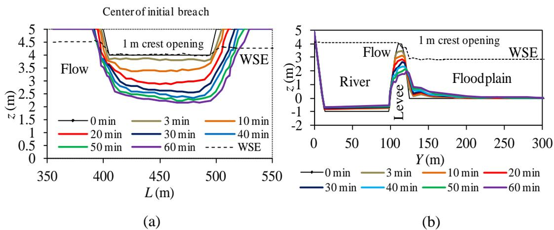
**Fig. 2.16** Evolution process of levee reach with time for  $Q=800 \text{ m}^3/\text{s}$ : (a) temporal growth of breaching section (front view at  $y=115 \text{ m}$ ); (b) temporal loss of levee cross section (side view at  $L=475 \text{ m}$ ).
