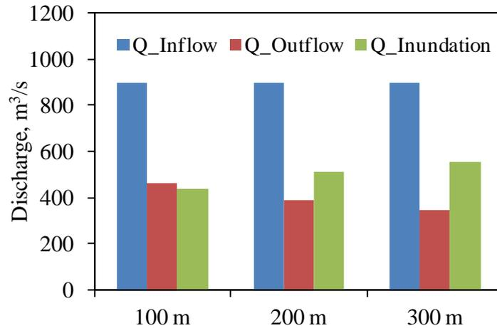
**Fig. 2.27** The river flow and the floodplain flow with various length of initial breach opening.
