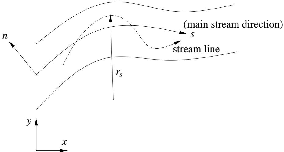
**Fig. 2.5** Definition sketch of streamline and radius of curvature ( $r_s$ )
