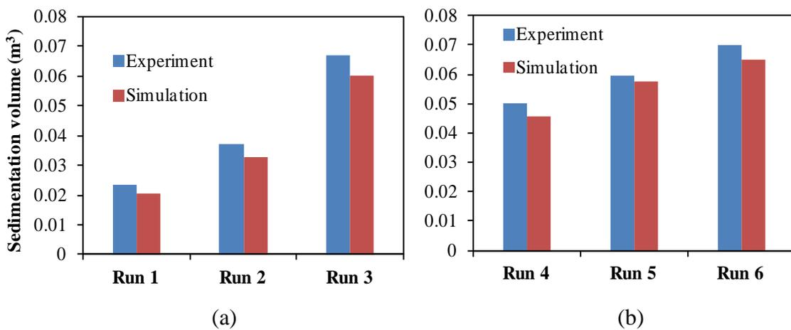
**Fig. 4.7** Comparisons of the volume of the floodplain sedimentation both in experiments and simulation Runs 1 to 6: (a) Coarser bed material and steep river bed slope; (b) Finer bed material and mild river bed slope.
