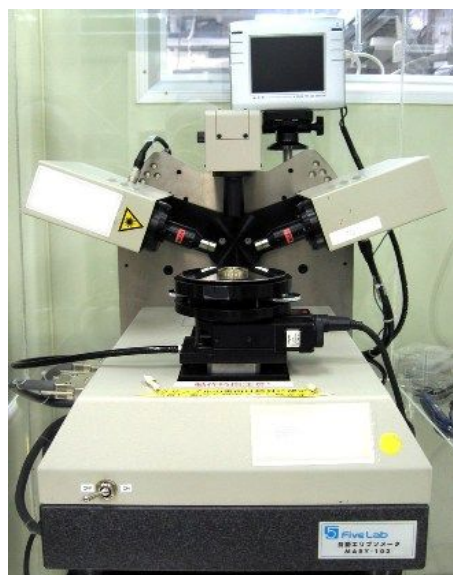
Fig. 3.7 Photograph of the scanning ellipsometer (MARY-102).
