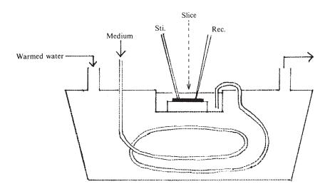
Fig. 2 Schematic drawing of the observation chamber. The slice mounted on the nylon net is perfused with oxygenated and warmed medium. Sti.: stimulating bipolar electrode; rec.: recording micropipette
