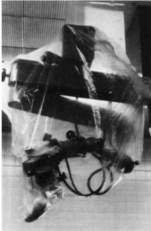
Fig. 1 Showing sterilization of ceiling type operating microscope.
