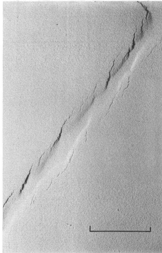
Fig. 2 Fault pattern on model surface illuminated at low angle from the left. Faults arranged en echelon are developed on either side of graben and fault throws diminish towards both ends of each fault.
