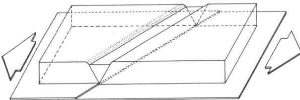
Fig. 1 Diagrammatic setup of graben experiment.
