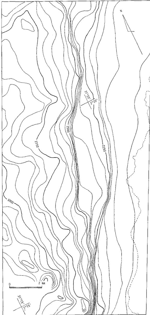
Fig. 6 Simplified topographic map of an area in Fig. 5 (contours: 50 feet intervals). Contour lines are smoothed out by burying valleys more than 1 km in width on topographic maps (scale; 1:50000).
