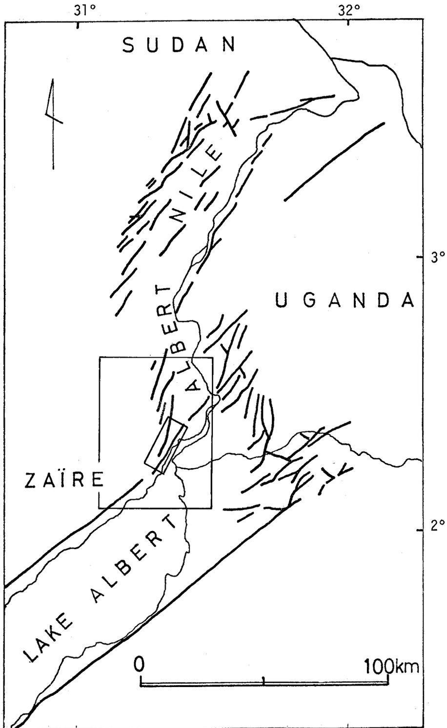
Fig. 4 Fault pattern in Albert Nile region. Faults are after MacDonald (1969) and the present work. Two squares in the map indicate localities of Fig. 5 and Fig. 6, respectively.
