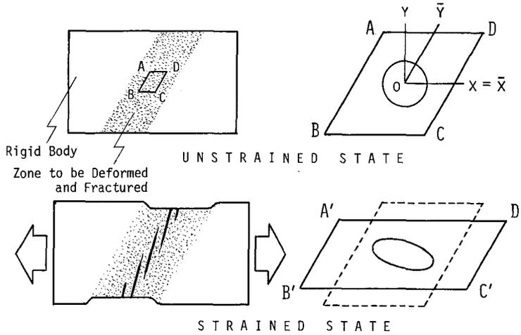
Fig. 2 Strain state of second order in a deformed zone.
