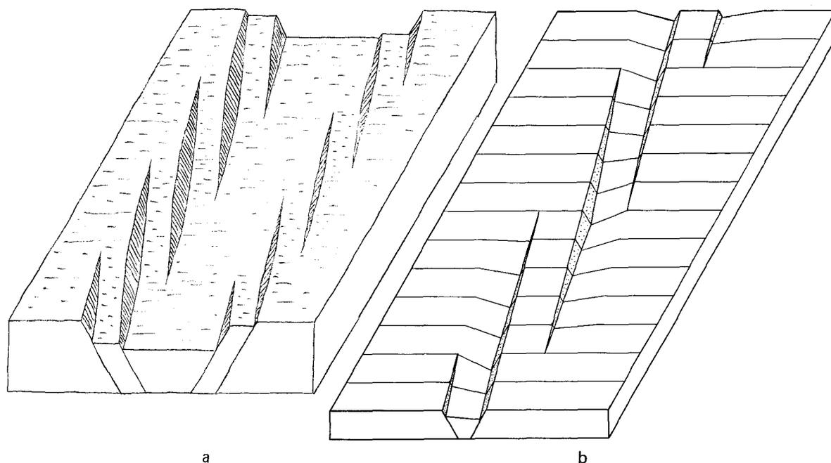
Fig. 3 Schematic model showing throw variation of normal faults arranged en echelon. a: en echelon faults developed on either side of graben. b: en echelon and overlapping graben structures.
