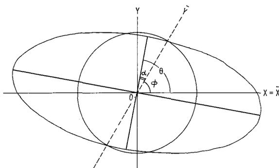
Fig. 4 Strain ellipse and RE-angle
